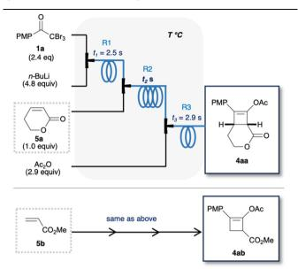
Reaction conditions: **1a** (2.4 equiv.,  $c_1$  = 0.10 mol L<sup>-1</sup>,  $v_1$  = 7.52 mL min<sup>-1</sup>, THF); n-BuLi (4.8 equiv.,  $c_2$  = 0.80 mol L<sup>-1</sup>,  $v_2$  = 1.88 mL min<sup>-1</sup>, n-hexane); 5 (1.0 equiv.,  $c_3$  = 0.12 mol L<sup>-1</sup>,  $v_3$  = 2.6 mL min<sup>-1</sup>, THF); Ac<sub>2</sub>O (2.9 equiv.,  $c_4$  = 0.23 mol L<sup>-1</sup>,  $v_4$  = 4.0 mL min<sup>-1</sup>, THF).  $t_1$  = 2.5 s,  $t_3$  = 2.9 s.
