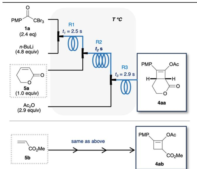
Reaction conditions: **1a** (2.4 equiv.,  $c_1 = 0.10 \text{ mol L}^{-1}$ ,  $v_1 = 7.52 \text{ mL min}^{-1}$ , THF); *n*-BuLi (4.8 equiv.,  $c_2 = 0.80 \text{ mol L}^{-1}$ ,  $v_2 = 1.88 \text{ mL min}^{-1}$ , *n*-hexane); **5** (1.0 equiv.,  $c_3 = 0.12 \text{ mol L}^{-1}$ ,  $v_3 = 2.6 \text{ mL min}^{-1}$ , THF);  $\text{Ac}_2\text{O}$  (2.9 equiv.,  $c_4 = 0.23 \text{ mol L}^{-1}$ ,  $v_4 = 4.0 \text{ mL min}^{-1}$ , THF).  $t_1 = 2.5 \text{ s}$ ,  $t_3 = 2.9 \text{ s}$ .
