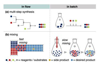
Fig. 1 Mechanical features in continuous flow and batch systems: (a) mass transfer in multi-step synthesis, (b) fast mixing in a flow system and slow mixing in a batch system.
