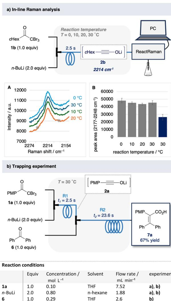
**Fig. 3** (a) In-line Raman analysis of **2b**. A: Observed Raman spectra, residence time = 2.5 s. B: peak area (2177–2248 cm<sup>-1</sup>), residence time = 2.5 s (grey bar), 22.5 s (blue bar). (b) Trapping experiment.
