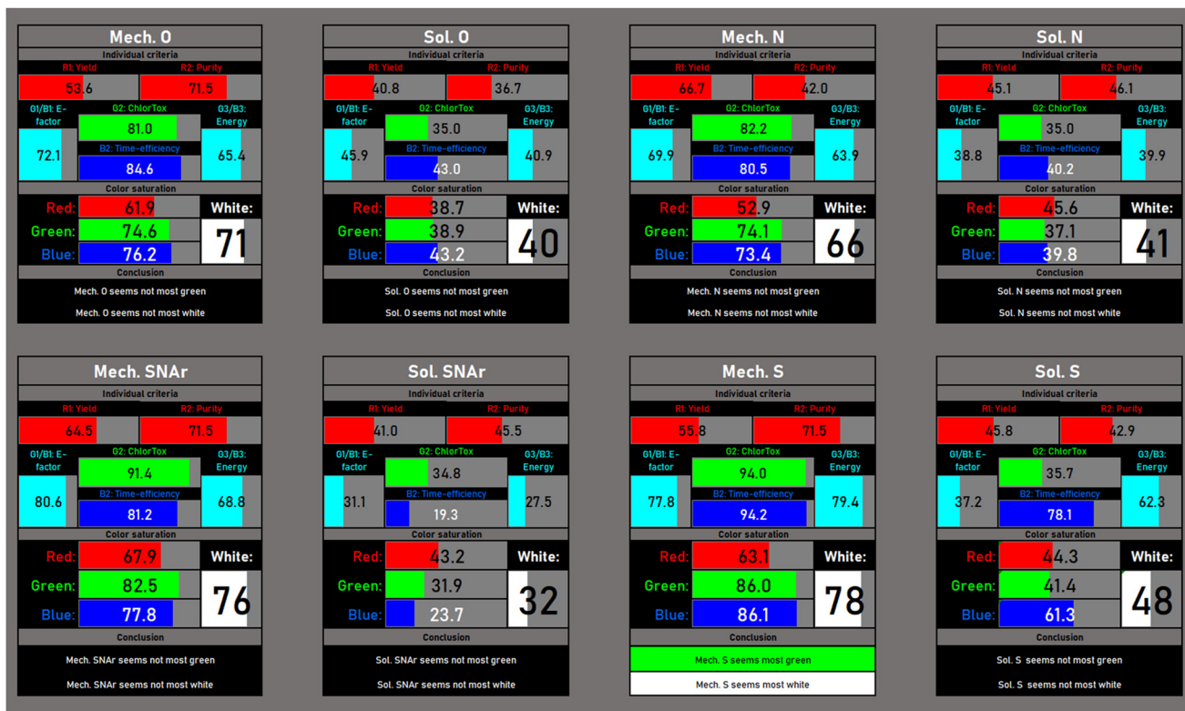
Fig. 6 Results of the assessment using the RGBsynt model for various types of synthesis carried out as mechanochemical (Mech.) and solution-based (Sol.) reactions, acquired as averaged values of the input data (each type of reaction included 4 or 5 unit procedures). The mechanochemical and solution-based procedures corresponded to the same products; O – O -alkylation, N – N -alkylation, SNAr – nucleophilic aromatic substitution, S – sulfonylation.
