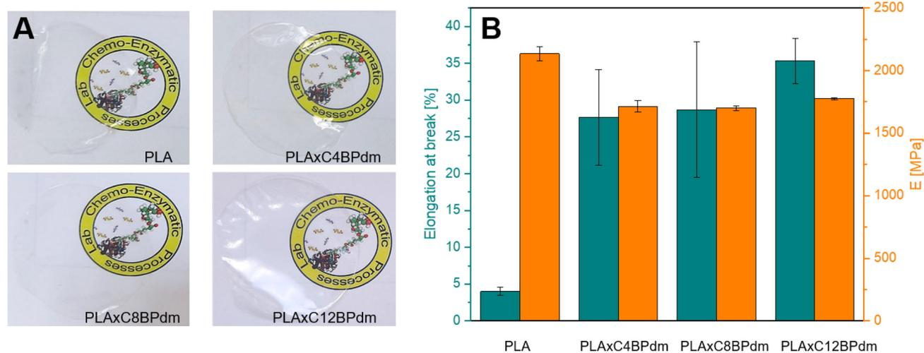
**Fig. 5** Mechanical characterization of the obtained blended PLA films. (A) Photos of PLA and PLA BPdm-containing films: neat PLA, PLAxC4BPdm, PLAxC8BPdm, and PLAx12BPdm. (B) Elongation at break ( $\epsilon_{\text{break}}$ ) and Young's modulus ( $E$ ) from the stress-strain test of PLA and PLA BPdm-containing films. Error bars represent the corresponding standard error.
