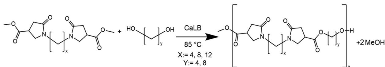
**Fig. 3** Reaction scheme of BPdm-based polycondensation. The reaction between BPdm structures spacers with  $x = [4, 8, 12]$  and a potentially bio-based diol with  $y = [4, 8]$  in a solventless enzymatically catalyzed reaction formed the BPdm-based oligomers. After 6 h at ambient pressure a further 18 h of reaction time at reduced pressure were applied.
