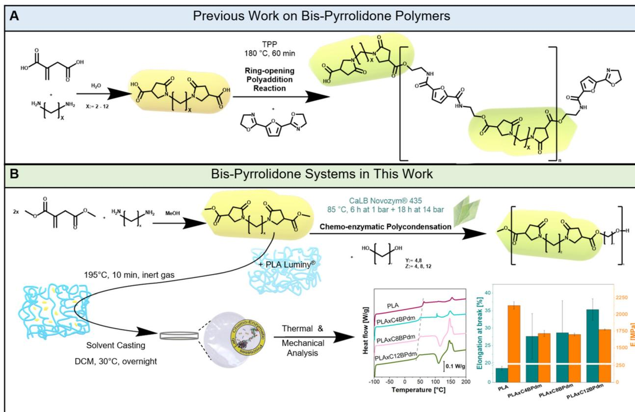
**Fig. 1** Scheme of the synthesis of bis-pyrrolidone (BP)-based polymers. (A) The BP-based polyaddition reaction previously reported by Roy *et al.* (mechanism adapted from Roy *et al.*, 2018)<sup>29</sup> and (B) the enzymatically synthesized CxBPdm-based polyester structure and poly(lactic acid) plasticization experiments carried out in this work. Representative graphs for mechanical and thermal analysis are given (see also Fig. 5, and Fig. S32 in the ESI†).
