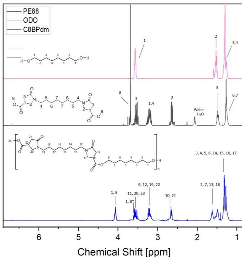
**Fig. 4**  $^1\text{H}$ -NMR spectra of polymer PE88 (blue) and monomers C8BPdm (black) and ODO (pink). The reported spectrum clearly shows the formation of the polyester as the  $-\text{OCH}_3$  signal (8 black) of the used C8BPdm monomer had a greatly reduced intensity in the final product while the intensity of the signal at 4.1 ppm ( $-\text{CH}_2-\text{CH}_2-\text{O}-\text{C}=\text{O}$ , 1,8 blue) increases.
