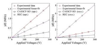
Fig. 2 The shift in transition frequency  $(\delta f)$  versus applied voltage V, showing a linear E-field coupling in  $HoW_{10}$ . Calculations correspond to the DFT-optimized structure (left) and to the crystallographic structure (right).  $^{51}$
