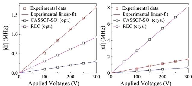
**Fig. 2** The shift in transition frequency ( $\delta f$ ) versus applied voltage  $V$ , showing a linear E-field coupling in  $\text{HoW}_{10}$ . Calculations correspond to the DFT-optimized structure (left) and to the crystallographic structure (right).<sup>51</sup>
