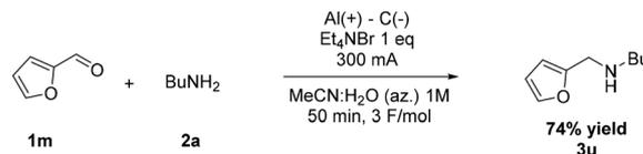
**Fig. 3** Electrochemical reductive amination on biomass-derived furfural. Reaction conditions: **1m** (3 mmol), **2a** (3 mmol), tetraethylammonium bromide (3 mmol), MeCN:H<sub>2</sub>O (az.) (3 mL), aluminium anode and graphite cathode, 300 mA until a 3 F mol<sup>-1</sup> charge is passed (ca. 50 minutes).
