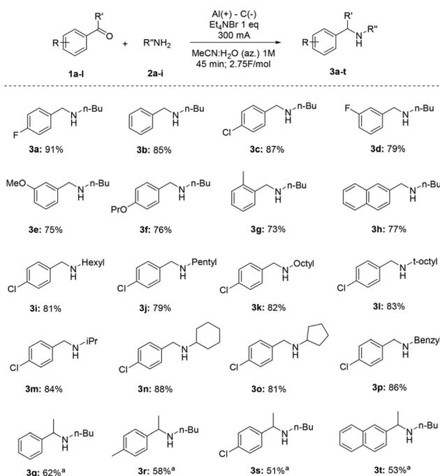
**Scheme 1** Substrate scope of ERA. Reaction conditions: **1a–l** (3 mmol), **2a–i** (3 mmol), tetraethylammonium bromide (3 mmol), MeCN:H<sub>2</sub>O (az.) (3 mL), 300 mA until a 2.75 F mol<sup>-1</sup> charge is passed (ca. 45 minutes). <sup>a</sup> Pre-step of imine formation is required. Products are isolated as hydrochloride salts.
