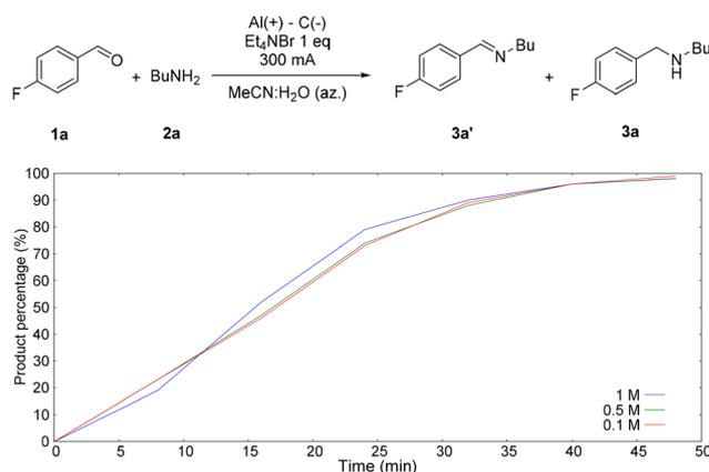
**Fig. 2** Reaction kinetics. Reaction conditions: **1a** (3 mmol), **2a** (3 mmol), tetraethylammonium bromide (3 mmol), 300 mA. Blue line: 1 M: MeCN : H<sub>2</sub>O (az.) (3 mL), samples taken every 8 minutes for up to 48 minutes of reaction. Green line: 0.5 M: MeCN : H<sub>2</sub>O (az.) (6 mL), samples taken every 8 minutes for up to 48 minutes. Red line: 0.1 M: MeCN : H<sub>2</sub>O (az.) (30 mL), samples taken every 8 minutes for up to 48 minutes.
