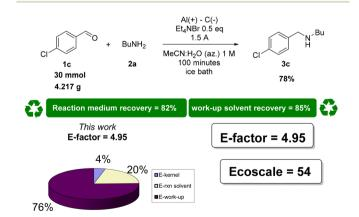
Scheme 2 Gram-scale ERA with solvent reclaims. Reaction conditions: 1c (30 mmol; 4.217 g), 2a (30 mmol; 2.194 g), tetraethylammonium bromide (15 mmol; 3.152 g), aluminium anode and graphite cathode, MeCN:  $H_2O$  (az.) (30 mL), 1.5 A, 100 minutes.
