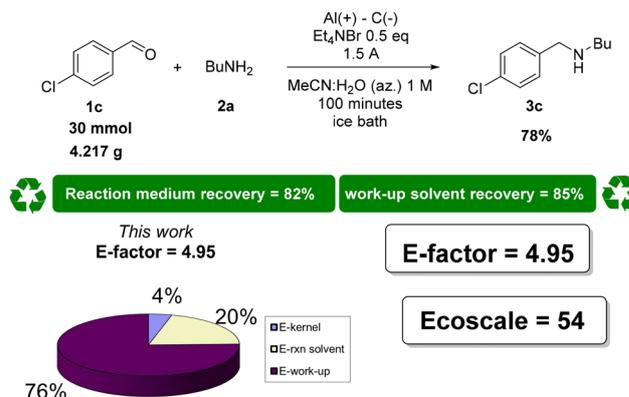
**Scheme 2** Gram-scale ERA with solvent reclaims. Reaction conditions: **1c** (30 mmol; 4.217 g), **2a** (30 mmol; 2.194 g), tetraethylammonium bromide (15 mmol; 3.152 g), aluminium anode and graphite cathode, MeCN:H<sub>2</sub>O (az.) (30 mL), 1.5 A, 100 minutes.
