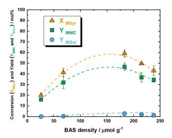
Fig. 2 Conversion of MSyr and yield of MMC and MGal over Beta zeolites as a function of BAS density. Reaction conditions: temperature: 210 °C, time: 2 h,  $N_2$  pressure = 1 bar, catalyst amount: 200 mg. BAS density: 26; 68; 183; 215; 238  $\mu$ mol  $q^{-1}$ .
