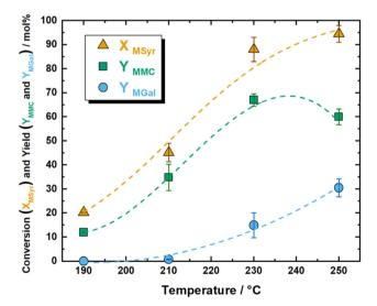
Fig. 4 Conversion of MSyr and yield of MMC and MGal over Beta 75 as a function of Temperature. Reaction conditions: time: 2 h,  $N_2$  pressure 1 bar, catalyst amount: 200 mg, temperature: 190 °C, 210 °C, 230 °C, and 250 °C.
