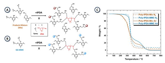
Fig. 7 Synthesis of (A) poly-IPDA-Mix and (B) poly-IPDA-MMC, see ESI† for the synthetic details. The blue and brown spheres indicate the repetition of the respective monomeric unit. (C) TGA in N2 (dashed line) and in air (full line) of the two prepared polymers.
