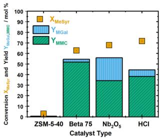
Fig. 1 Conversion of MSyr ( $X_{MSyr}$ ) and yield of MMC and M-Gal yield ( $Y_{MMC}$  and  $Y_{MGal}$ ) as a function of different used acid catalysts. Reaction conditions for heterogeneous catalysts: temperature: 210 °C, time: 4 h,  $N_2$  pressure = 1 bar, catalyst amount: 200 mg. Reaction conditions for HCl: temperature: 250 °C, time: 1 hour,  $N_2$  pressure = 46 bar- to ensure HCl in liquid state, catalyst amount: 1.45 mmol HCl.
