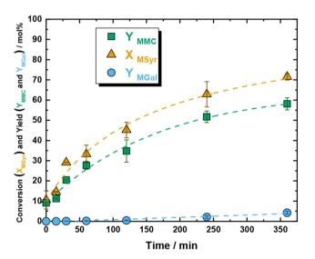
Fig. 3 Conversion of MSyr and yield of MMC and MGal over Beta 75 as a function of time. Reaction conditions: time: 0 min, 15 min, 30 min, 60 min, 120 min, 240 min, 360 min,  $N_2$  pressure 1 bar, catalyst amount: 200 mg, temperature: 210 °C.
