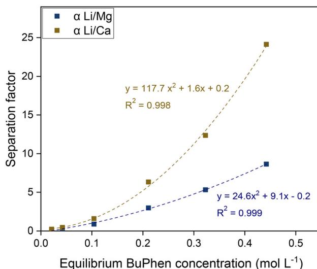
Fig. 5 Separation factors  $\alpha_{\text{Li/Mg}}$  and  $\alpha_{\text{Li/Ca}}$  as a function of the equilibrium BuPhen concentration for 0.050 mol L<sup>-1</sup> saponified D2EHDTPA diluted in *n*-dodecane with 10 vol% 1-octanol and 2-octanol. The aqueous phase contained 0.050 mol L<sup>-1</sup> each of LiCl, KCl, RbCl, MgCl<sub>2</sub> and CaCl<sub>2</sub>. Phase volume ratio: 1:1, equilibrium temperature: 25 °C.
