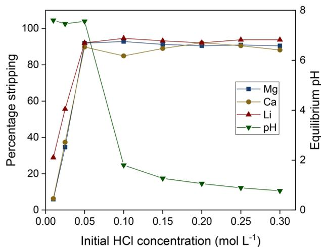
Fig. 12 Stripping of lithium, magnesium and calcium from a loaded organic phase consisting of saponified D2EHDTPA ( $0.050 \text{ mol L}^{-1}$ ), BuPhen ( $0.250 \text{ mol L}^{-1}$ ), 2,5 vol% 1-octanol and 20 vol% 2-octanol in *n*-dodecane, loaded from a solution of LiCl,  $\text{MgCl}_2$  and  $\text{CaCl}_2$  ( $0.050 \text{ mol L}^{-1}$  each). Phase volume ratio: 1 : 1, equilibrium temperature:  $25^\circ \text{C}$ .
