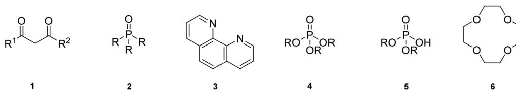
**Fig. 1** Structures of reported extractants for lithium solvent extraction. 1:  $\beta$ -Diketone. 2: Trialkylphosphine oxide. 3: 1,10-Phenanthroline. 4: Trialkyl phosphate. 5: Dialkylphosphoric acid. 6: Crown ether.
