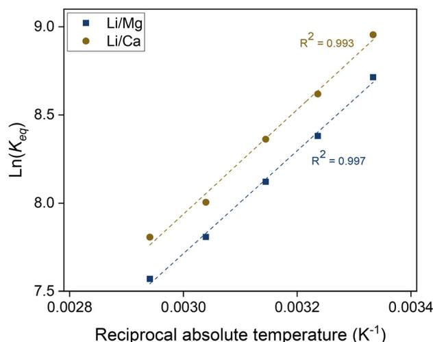
**Fig. 11** Van't Hoff plot of the ion-exchange reactions between lithium and magnesium and between lithium and calcium. Organic phase: 0.050 mol L<sup>-1</sup> of D2EHDTPA saponified with LiOH, 0.125 mol L<sup>-1</sup> of BuPhen, 2.5 vol% 1-octanol, 20 vol% 2-octanol, diluted in *n*-dodecane. Aqueous phase: 0.050 mol L<sup>-1</sup> each of MgCl<sub>2</sub> and CaCl<sub>2</sub>. Phase volume ratio: 1 : 1.
