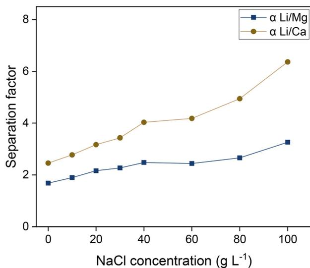
**Fig. 9** Influence of the NaCl concentration on the separation factors. Organic phase: 0.050 mol L<sup>-1</sup> of saponified D2EHDTPA 0.125 mol L<sup>-1</sup> of BuPhen, 2.5 vol% 1-octanol, 20 vol% 2-octanol, diluted in *n*-dodecane. Aqueous phase: 0.050 mol L<sup>-1</sup> each of LiCl, MgCl<sub>2</sub> and CaCl<sub>2</sub>, and a variable NaCl concentration. Phase volume ratio: 1 : 1, equilibrium temperature: 25 °C.
