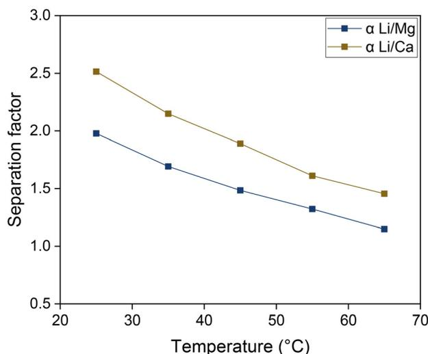
**Fig. 10** Influence of the equilibrium temperature on the separation factors. Organic phase: 0.050 mol L<sup>-1</sup> of D2EHDTPA saponified with LiOH, 0.125 mol L<sup>-1</sup> of BuPhen, 2.5 vol% 1-octanol, 20 vol% 2-octanol, diluted in *n*-dodecane. Aqueous phase: 0.050 mol L<sup>-1</sup> each of MgCl<sub>2</sub> and CaCl<sub>2</sub>. Phase volume ratio: 1 : 1.
