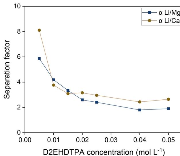
**Fig. 8** Influence of the saponified D2EHDTA concentration on the separation factors. Organic phase: 0.125 mol L<sup>-1</sup> of BuPhen, 2.5 vol% 1-octanol, 20 vol% 2-octanol, diluted in *n*-dodecane. Aqueous phase: 0.050 mol L<sup>-1</sup> each of MgCl<sub>2</sub> and CaCl<sub>2</sub>, 50 g L<sup>-1</sup> of NaCl, and equimolar LiCl with respect to D2EHDTA. Phase volume ratio: 1:1, equilibrium temperature: 25 °C.
