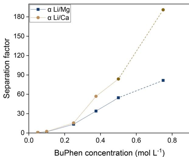
**Fig. 7** Influence of the BuPhen concentration on the separation factors. Organic phase: 0.05 mol L<sup>-1</sup> saponified D2EHDTA, 2.5 vol% 1-octanol (5 vol% for 0.750 mol L<sup>-1</sup> BuPhen), 20 vol% 2-octanol, diluted in *n*-dodecane. Aqueous phase: 0.050 mol L<sup>-1</sup> each of LiCl, KCl, RbCl, MgCl<sub>2</sub> and CaCl<sub>2</sub>. Phase volume ratio: 1:1, equilibrium temperature: 25 °C.
