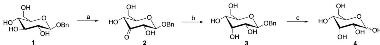
**Scheme 1** Chemo-enzymatic synthesis of D-allose from 1-*O*-benzyl- $\beta$ -glucopyranoside. (a) 1 U ml<sup>-1</sup> of 16F10 enzyme, 0.1 mg ml<sup>-1</sup> of catalase at pH 7.5, 25 °C for 6 h30 min under aerobic conditions, 100% yield; (b) LS-Selectride, DMSO : THF (2 : 1), 0 °C, 2 h, 86%; (c) Pd/C 10%, 50 psi, MeOH, overnight, 94%.
