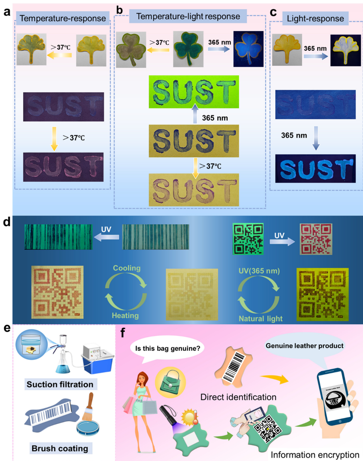
Fig. 8 Ginkgo biloba , clover, SUST shape temperature-response (a), temperature–light double response (b), and light-response (c) leather anti-counterfeiting pattern. (d) Temperature–light response leather barcode, and QR code anti-counterfeiting pattern. (e) The production method of the leather anti-counterfeiting pattern. (f) Application scenario diagram of leather anti-counterfeiting patterns.
