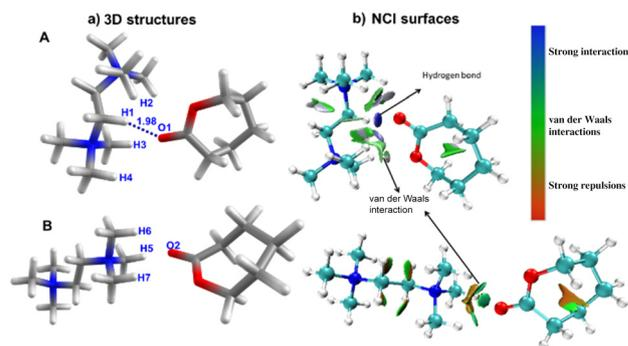
**Fig. 5** (a) Molecular modelling of complexes between the cationic catalyst and  $\epsilon$ -CL in different orientations of these species (**A** and **B**) (b) NCI surfaces (iso value = 0.5). Color code: C (black), O (red), H (grey), and N (blue).
