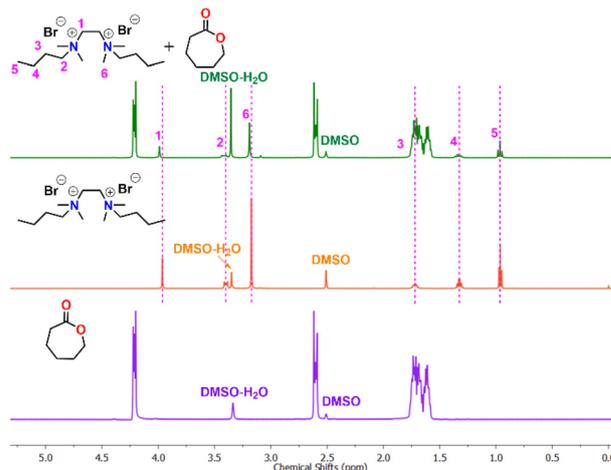
Fig. 3 <sup>1</sup>H NMR spectra of complex formed *in situ* in the mixture of salt **1** and  $\epsilon$ -CL in DMSO.
