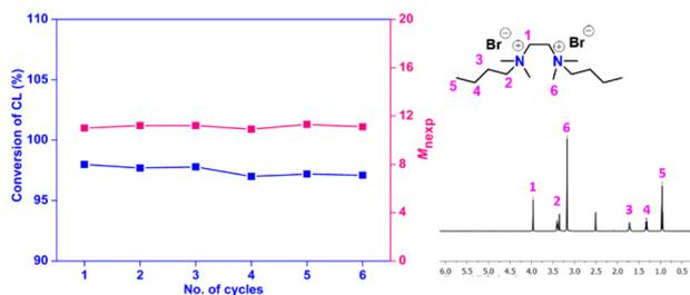
**Fig. 6** (a) Recycling studies of *N,N'*-dibutyl-*N,N,N',N'*-tetramethylethane-1,2-diammonium bromide as the catalyst for the ROP of  $\epsilon$ -CL and (b)  $^1\text{H}$  NMR spectra of the catalyst after 6th cycle.
