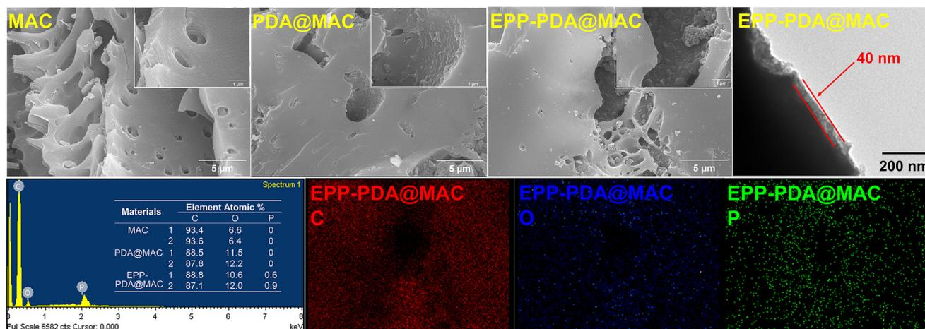
Fig. 2 SEM and TEM micrographs, EDS spectra, elemental mapping images of MAC, PDA@MAC, and EPP-PDA@MAC.
