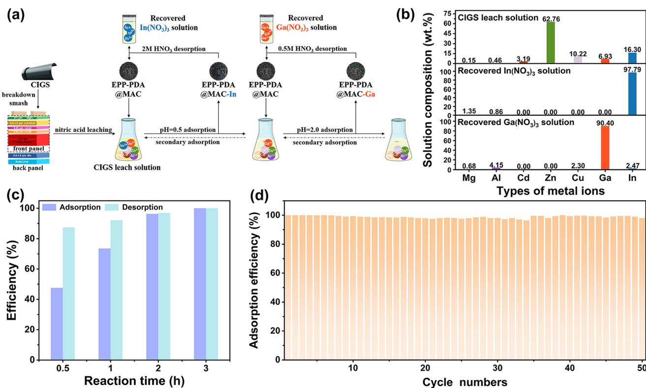
Fig. 6 (a) The application of EPP-PDA@MAC for the recovery of  $\text{In}^{3+}$  and  $\text{Ga}^{3+}$  from waste CIGS photovoltaic modules. (b) The composition of the CIGS leach solution and recovered  $\text{In}(\text{NO}_3)_3$  and  $\text{Ga}(\text{NO}_3)_3$  solutions. (c) Effect of the reaction time on adsorption and desorption, and (d) the number of cycles of EPP-PDA@MAC in the CDI system.
