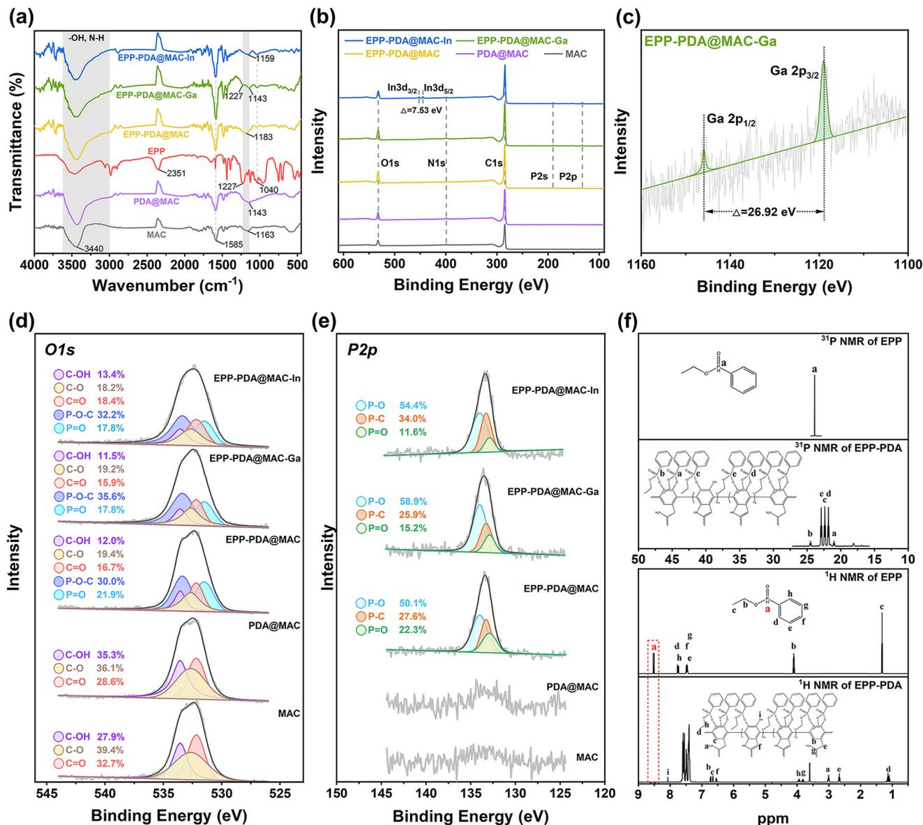
Fig. 4 (a) FT-IR spectra, (b and c) XPS spectra, (d) O 1s, and (e) P 2p spectra of the MAC, PDA@MAC, EPP, EPP-PDA@MAC, and EPP-PDA@MAC-In/Ga. (f) <sup>1</sup>H-NMR and <sup>31</sup>P-NMR spectra of EPP and EPP-PDA.
