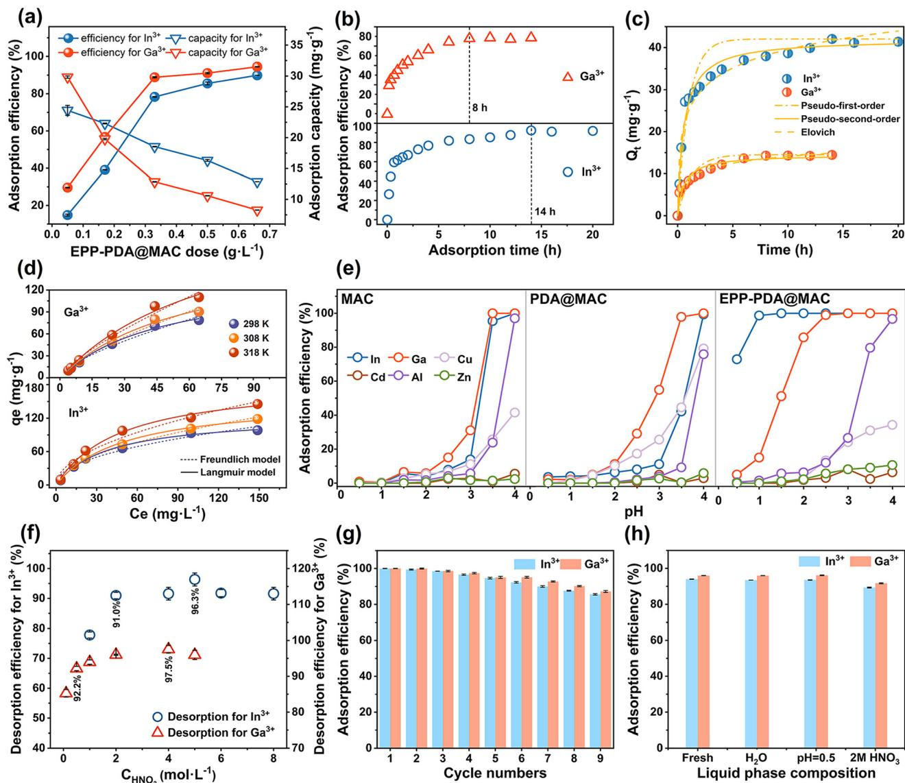
**Fig. 3** Effect of (a) dose and (b) reaction time on the adsorption efficiency. (c) Kinetic and (d) isotherm fitting models for adsorption. (e) Adsorption efficiency for different ions in mixed solutions at pH 0.5–4. (f) Effect of nitric acid concentration on the desorption efficiency of  $\text{In}^{3+}$  and  $\text{Ga}^{3+}$ . (g) Number of cycles of EPP-PDA@MAC in the static system. (h) Effect of the liquid phase composition on the adsorption ability after leaching treatment.
