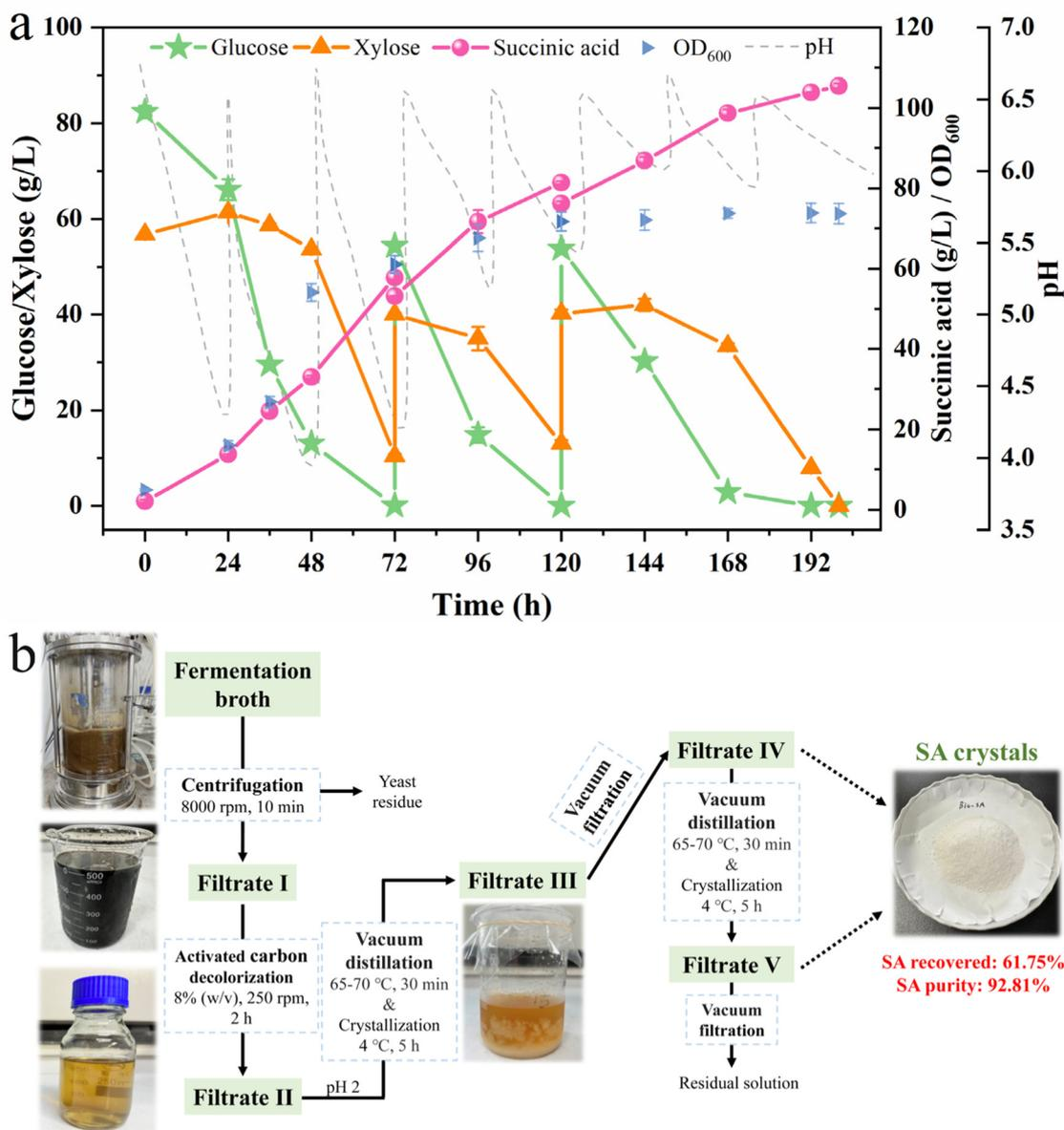
Fig. 6 Fed-batch fermentation of *Y. lipolytica* BDic5 in a 3 L bioreactor with undetoxified DLCA(sa)-CS hydrolysate (a), and the modified procedures for recovery of SA from acidic fermentation broth (b).
