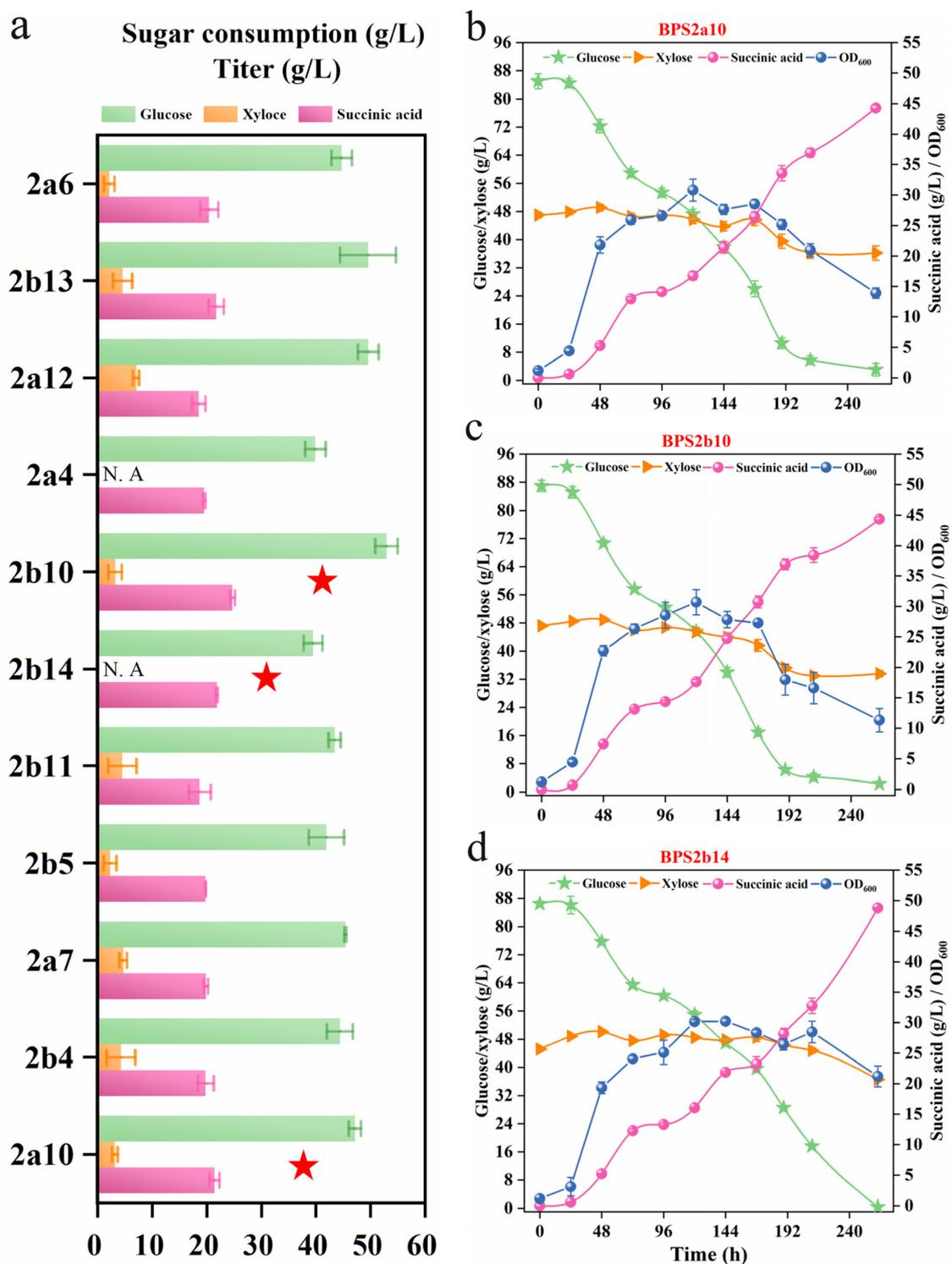
**Fig. 3** Comparison of sugar consumption and SA production of randomly selected transformants (a), and long-term shaking flask fermentation of preponderant strains BPS2a10 (b), BPS2b10 (c), and BPS2b14 (d). The initial concentrations of glucose and xylose were approximately 80 and 40 g L<sup>-1</sup>, respectively. The red star symbol represents the transformants with comparatively enhanced fermentation performance.
