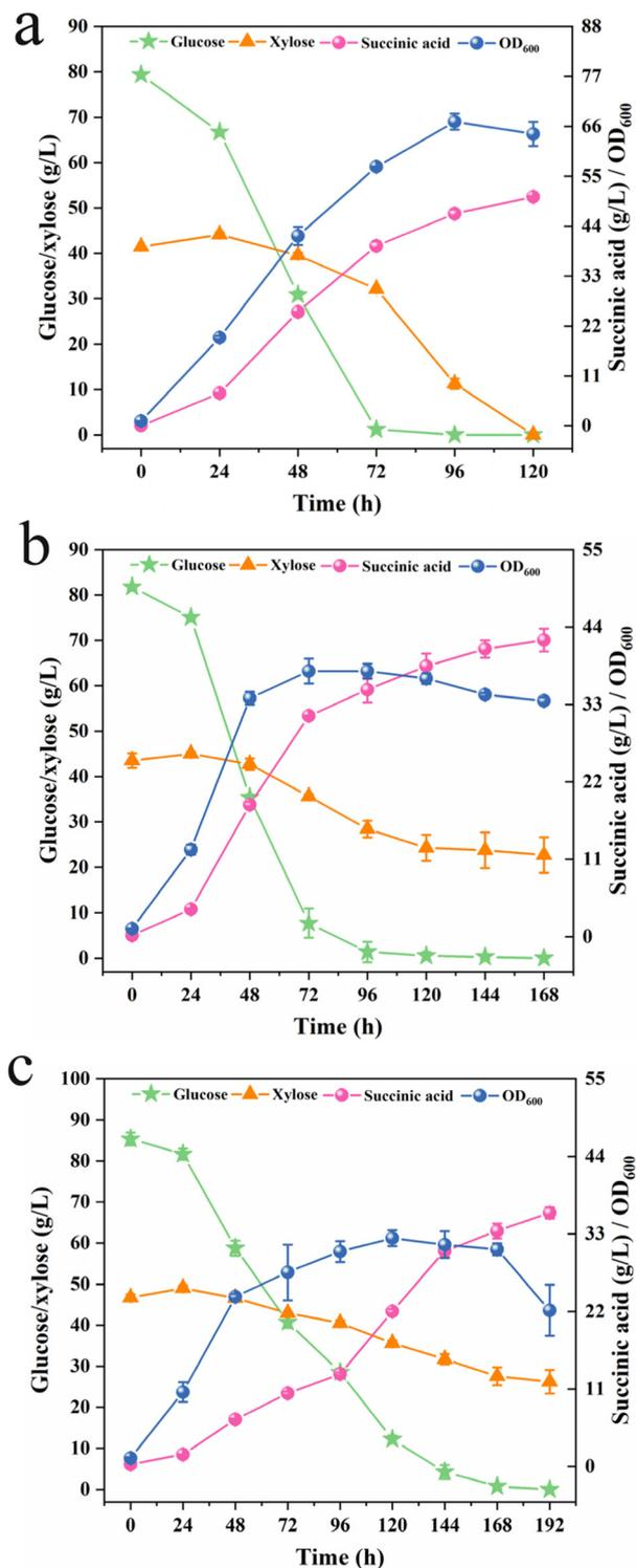
**Fig. 4** Effect of overexpression of transporters on sugar assimilation rate and SA production: mitochondrial dicarboxylic acid transporter *YIDic* (a), C4-dicarboxylic acid transporter *YIMae* (b), and combined overexpression of *YIDic* and *YIMae* (c).
