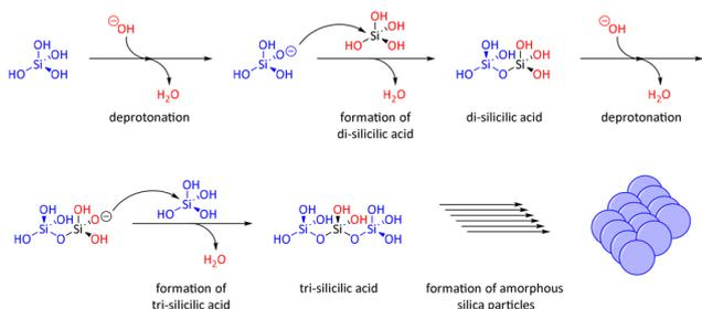
Fig. 18 Schematic representation of the S<sub>N2</sub>-like mechanism of silicic acid polycondensation that eventually leads to amorphous silica particle formation.
