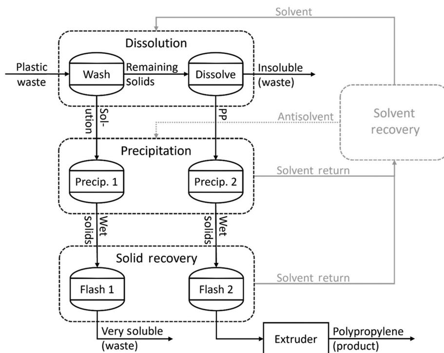
**Fig. 1** Generic process diagram of the PP-targeted solvent-based recycling process. Vessels in the dissolution and precipitation sections are jacketed pressure vessels. Flash vessels in the solid recovery section are preceded by heaters.
