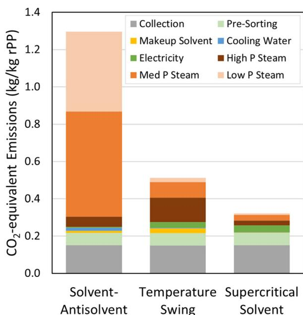
Fig. 3 CO<sub>2</sub>-equivalent emissions for the three base-case solvent-based processes.
