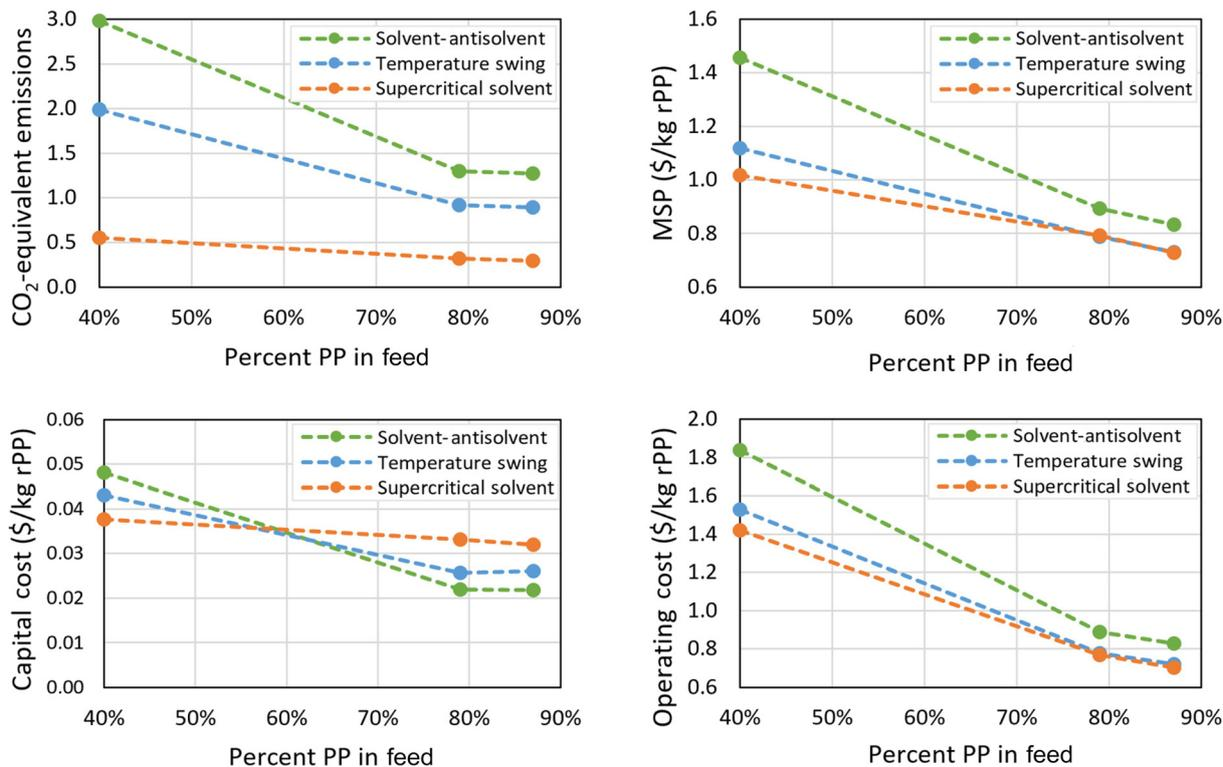
Fig. 7 CO<sub>2</sub>-equivalent emissions, MSP, and distributed CAPEX and OPEX for solvent-based recycling processes with varying feed compositions.
