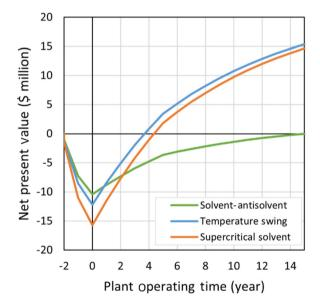
Fig. 5 NPV of the three base-case solvent-based processes.
