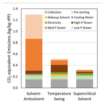
Fig. 3 CO<sub>2</sub>-equivalent emissions for the three base-case solvent-based processes.
