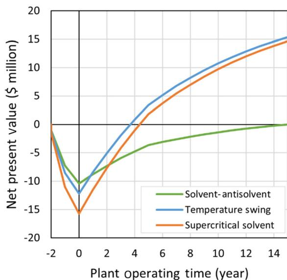
Fig. 5 NPV of the three base-case solvent-based processes.
