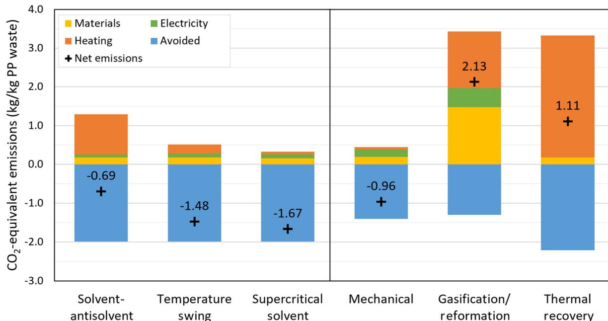
Fig. 6 Comparison of CO<sub>2</sub>-equivalent emissions for six PP treatment routes. Mechanical, gasification, and thermal routes are based on the processes described in the literature with updated emission factors.
