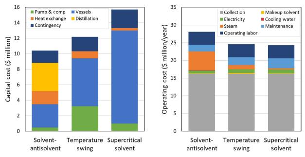
Fig. 4 Capital and operating costs for the three base-case solvent-based processes.
