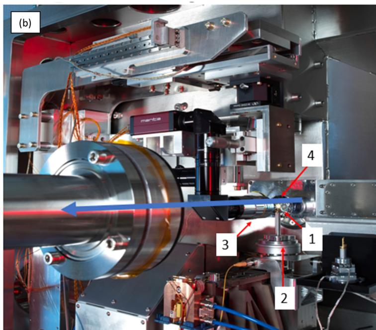
**Fig. 1** (a) A schematic of the I14 hard X-ray nanoprobe beamline layout showing the major components. (b) Inside the I14 hard X-ray nanoprobe experimental hutch showing the endstation, the blue arrow indicates the X-ray beam direction. 1–4 show the position of the (1) sample mounting position, (2) scanning and rotation stages, (3) sample alignment microscope, and (4) four-element silicon drift detector (XRF detector).
