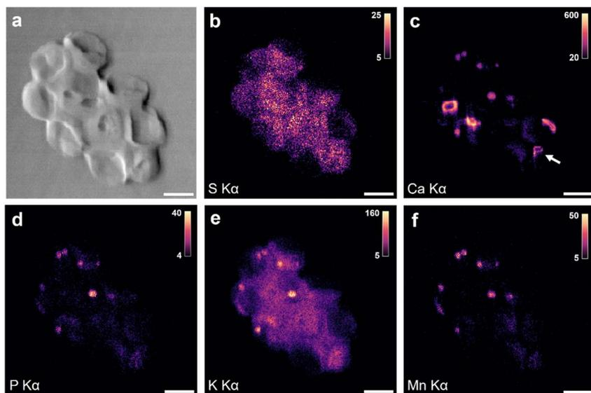
Fig. 3 A cluster of dried EDTA-treated *G. huxleyi* cells shown with (a) X-ray phase contrast imaging, (b) S  $K\alpha$  XRF, (c) Ca  $K\alpha$  XRF, (d) P  $K\alpha$  XRF, (e) K  $K\alpha$  XRF, and (f) Mn  $K\alpha$  XRF. Intensity scale shown as XRF counts. A logarithmic-base intensity scale is used for (c). Arrow in (c) points to proto-coccolith. Scale bar 3  $\mu\text{m}$ .
