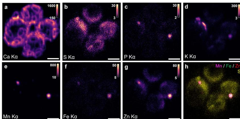
Fig. 2 Nano-XRF analysis of dried, coccolith-bearing *G. huxleyi* showing (a) Ca  $K\alpha$  XRF, (b) S  $K\alpha$  XRF, (c) P  $K\alpha$  XRF, (d) K  $K\alpha$  XRF, (e) Mn  $K\alpha$  XRF, (f) Fe  $K\alpha$  XRF, and (g) Zn  $K\alpha$  XRF maps. (h) Composite map of Mn, Fe, Zn, and S XRF signals. Intensity scale shown as XRF counts. Scale bar 2  $\mu\text{m}$ .
