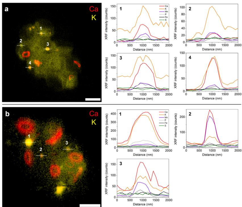
Fig. 5 Composite maps of Ca and K XRF for (a) EDTA-decalcified *G. huxleyi* and (b) early-stage recalcifying *G. huxleyi*. Inspected ion-rich bodies are numbered along with a horizontal dotted line that indicates the pixels used to create XRF intensity line profile plots found beside each composite map. Scale bar 3 μm.
