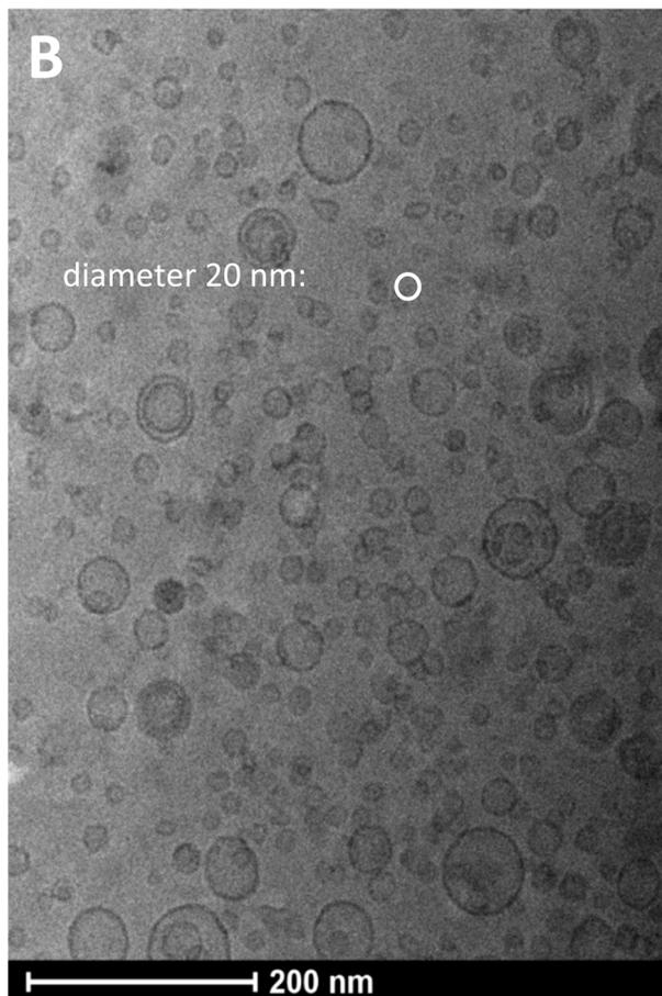
Fig. 4 Detection of small DVs in aLUV prepared at  $15^\circ\text{C}$  after cyclodextrin removal and subsequent temperature increase as seen by AF4 (A) and cryo-transmission electron microscopy (cryo-TEM) (B). (A) The red dash-dot line (fluorescence signal, left axis) and black dots (MALS, right axis) represent a sample with 23 mol% DPPG in the outer leaflet after 30 min incubation at  $35^\circ\text{C}$ , measured at  $23^\circ\text{C}$ . The grey dashed curve (left axis) and
