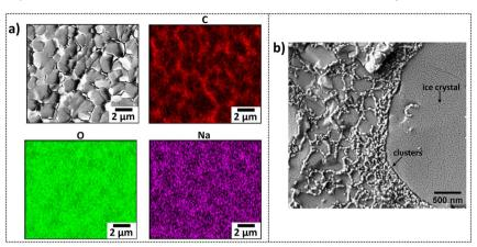
Fig. 6 (a) Elemental mapping by EDX spectroscopy of a slush frozen, hydrated, folded BSA hydrogel (7.4% BSA) prepared ex situ prior to freezing. Assigned elements are labelled on top of each image. (b) High magnification cryo-SEM image of the same hydrogel displaying a network wall structure of interconnected clusters that have been displaced to the boundaries of the ice filled pores.
