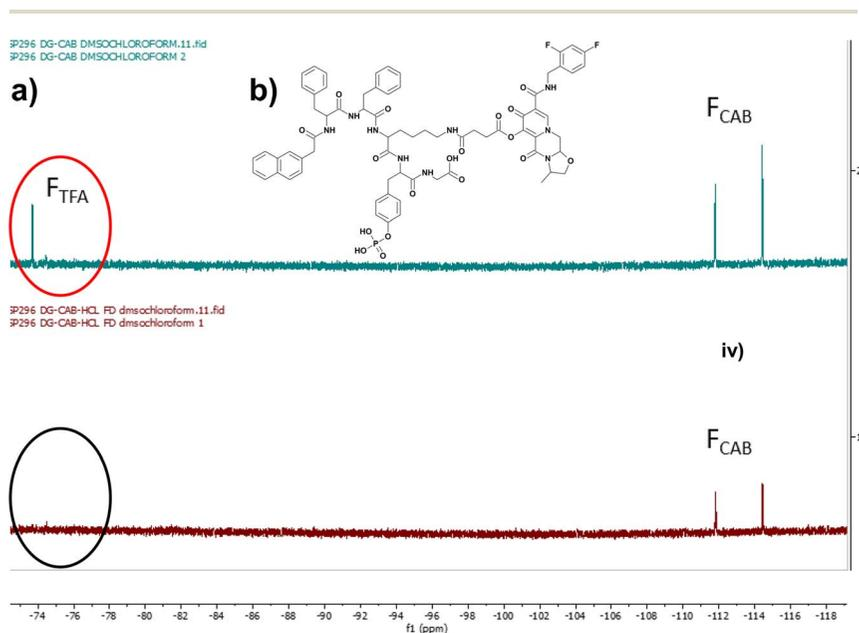
Fig. 1 (a) <sup>19</sup>F NMR demonstrates that removal of TFA was achieved by three repeated cycles of dissolving peptide in 5 mM HCl and freeze-drying. Monitoring shows removal of the singlet fluorine peak associated with TFA at  $-75$  ppm (circled red, black circle shows removal). Key:  $F_{TFA}$  <sup>19</sup>F NMR peaks associated with fluorine in TFA (red circle);  $F_{CAB}$  <sup>19</sup>F NMR peaks associated with fluorine in cabotegravir. (b) Chemical structure of Napffk(CAB)y(p)G-OH.
