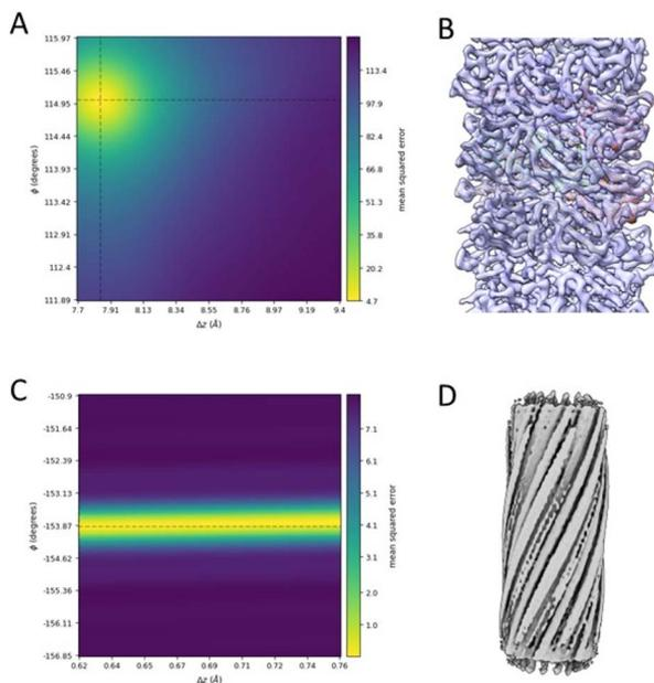
Fig. 4 Helical symmetry error surface plots and resultant maps generated by the Helix refine job in cryoSPARC for (A and B) *E. coli* Type 1 pili, and (C and D) the CarbIF micelle. The local search for symmetry was enabled at 6 Å for both cases. While symmetry parameters for Type 1 pili converged well, resulting in a high-resolution map, the convergence for the CarbIF micelle failed.
