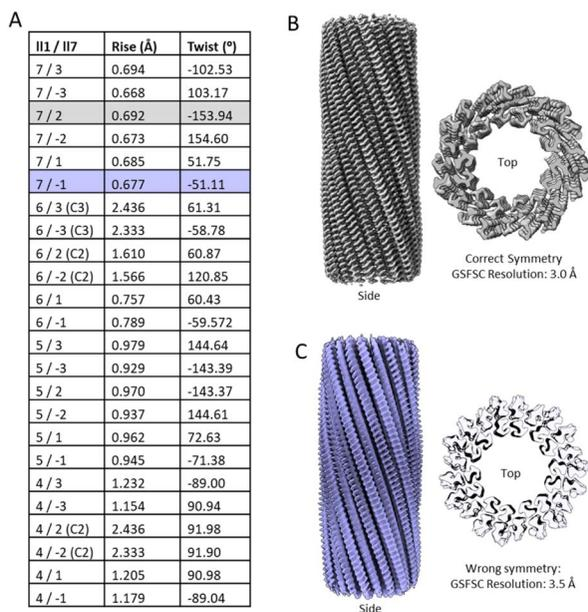
**Fig. 3** (A) Possible helical symmetry parameters for the CarbIF micelle calculated from the power spectrum shown in Fig. 1(D).  $C_n$  in parentheses indicates the relevant point group symmetry if one is present. (B and C) Cryo-EM maps of CarbIF generated by imposing the correct (B) and wrong (C) symmetry parameters. Strands are separated in both maps, while the peptide backbone within a strand is resolved well only in the correct map.
