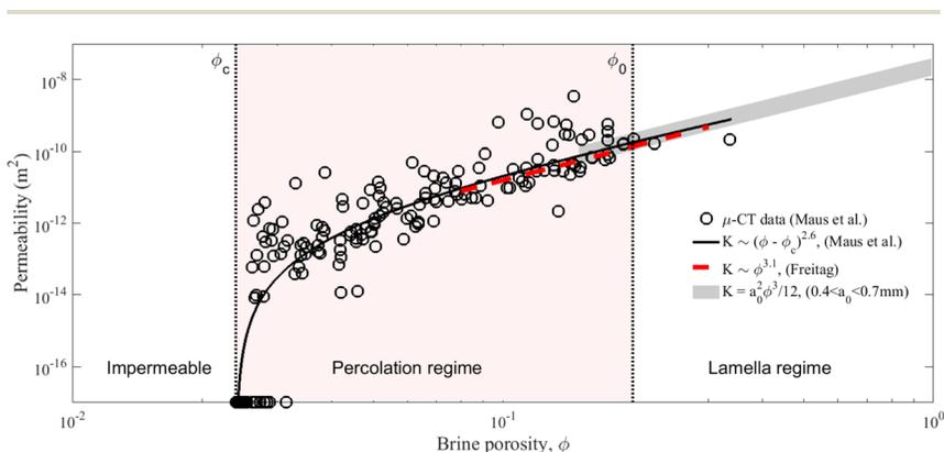
Fig. 1 Vertical permeability simulations *versus* brine porosity with best columnar ice fit from Maus *et al.*<sup>21</sup> compared to the relationship obtained by Freitag<sup>24</sup> for young ice (red curve), and the lamella model at high porosity (eqn (5)) for a typical range in sea ice plate spacing). The regime boundary for  $\phi_0$  described in the text is chosen tentatively.
