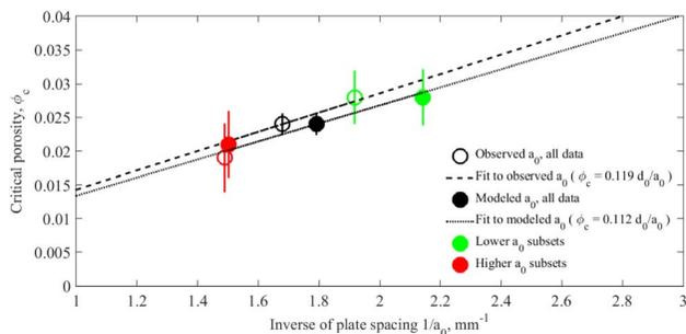
Fig. 8 Inverse measured and observed plate spacings  $a_0^{-1}$  versus the average percolation threshold  $\phi_c$  obtained by drawing model curves through each permeability simulation point for all data and for subgroups of high and low growth rate (low and high  $a_0$ ). The slope of the lines is  $d_0\phi_c$ .
