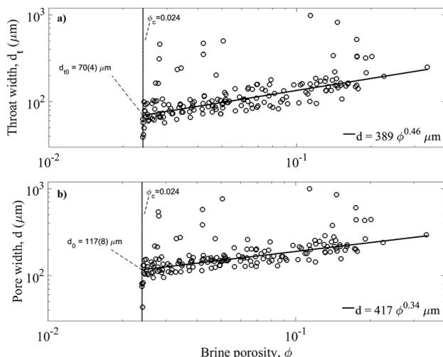
Fig. 5 (a) Median throat width  $d_t$  versus brine volume of young ice from ref. 21; (b) median pore diameter  $d$ . The critical  $d_{t0}$  and  $d_0$  values are obtained at the intersection of the relationships with the percolation threshold  $\phi_c$ .
