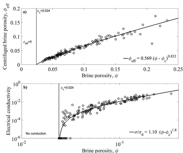
**Fig. 6** (a) Centrifuged (effective, open) brine porosity of young ice with optimum percolation fit from ref. 21; (b) normalised electrical conductivity with optimum percolation fit against  $(\phi - \phi_c)$  (new result).
