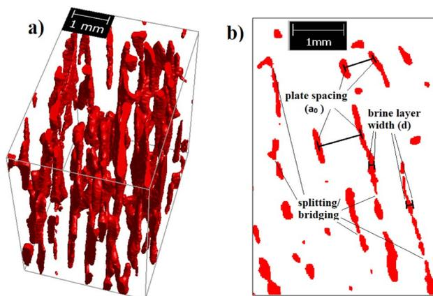
Fig. 2 3D (a) and 2D (b) micro-CT-based images of open pores in young sea ice, illustrating the plate (or brine layer) spacing  $a_0$ , the width  $d$  and the locations where the layer has split/bridged.
