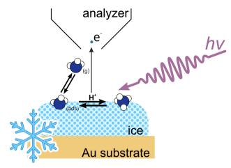
Fig. 1 Schematic of NH<sub>3</sub> adsorption at the ice-vapor interface in our experimental setup.
