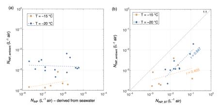
Fig. 11 Comparisons between ambient  $N_{\rm INP}$  measured from impinger samples and coincident  $N_{\rm INP}$  measured from (a) seawater and (b) BT-aerosol filters. The dashed lines indicate the linear regression in the logarithmic scale, and only the statistically significant (p < 0.05) r values (correlation coefficients) are shown in the figure. The correlation coefficients of all data are given in Table A1.†
