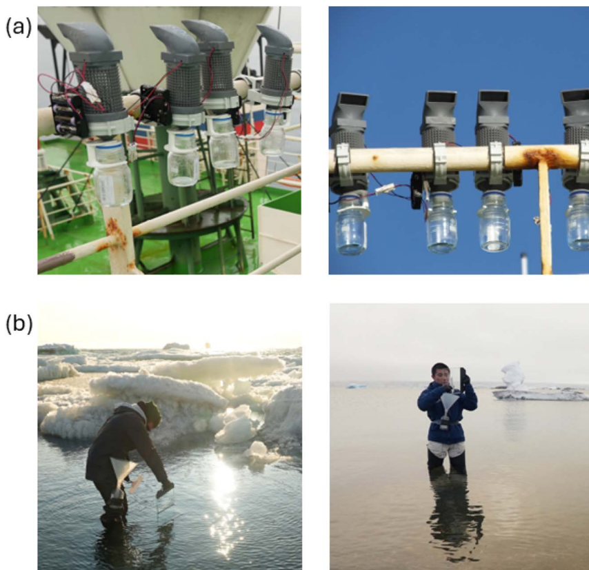
Fig. 3 (a) Fog water sample collector; (b) collection of SML.
