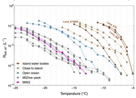
Fig. 8 Cumulative INP spectra for BT-generated particles, classified according to the sampling location. "Island water bodies" indicates water collected from island rivers and lakes, "MilliQ" denotes a reference experiment with pure water. All other categories are seawater samples. "Close to island" indicated that the ship location was less than 15 km from the coastline.
