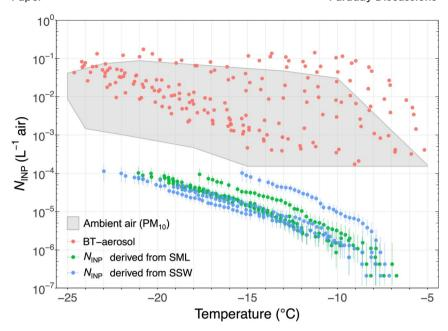
Fig. 9 Atmospheric  $N_{\text{INP}}$  as a function of temperature measured from ambient air by LVS filter with the PM<sub>10</sub> inlet (gray shaded area), BT-aerosol collected on filters (red), and  $N_{\rm INP}$ derived from SML (green) and SSW (blue) samples, respectively. The factor used to convert  $N_{\rm INP}$  in the SML and SSW samples to concentration in air is  $10^{-10.53}$
