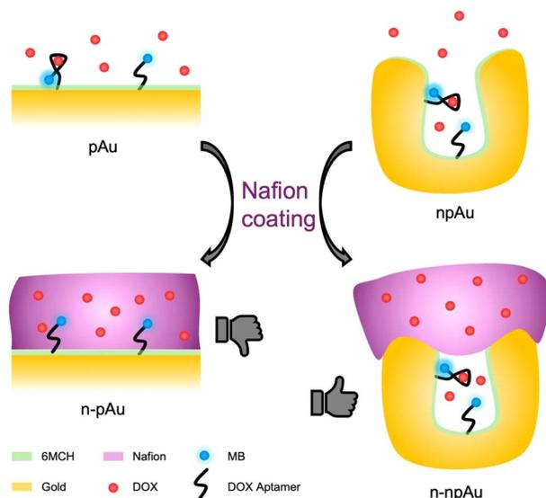
**Scheme 1** Schematic illustrations of Nafion-coated planar gold (n-pAu) electrode and Nafion-coated nanoporous gold (n-npAu) electrode for electrochemical aptamer-based biosensing. Nafion blocks the aptamer from changing conformation in the case of n-pAu, while the aptamer retains its redox signal change upon target binding in the case of n-npAu.
