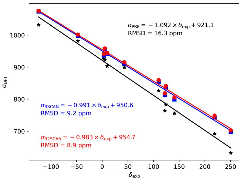
Fig. 4  $^{35/37}\text{Cl}$  magnetic shieldings,  $\sigma$ , calculated with the PBE (black), rSCAN (blue) and r<sup>2</sup>SCAN (red) functionals vs. experimental chemical shifts,  $\delta$ . For each functional the line of best fit is given.
