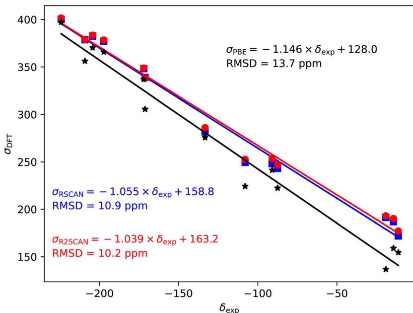
Fig. 2 <sup>19</sup>F magnetic shieldings,  $\sigma$ , calculated with the PBE (black), rSCAN (blue) and r<sup>2</sup>SCAN (red) functionals vs. experimental chemical shifts,  $\delta$ . For each functional the line of best fit is given.
