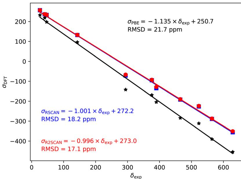
Fig. 3  $^{17}\text{O}$  magnetic shieldings,  $\sigma$ , calculated with the PBE (black), rSCAN (blue) and r<sup>2</sup>SCAN (red) functionals vs. experimental chemical shifts,  $\delta$ . For each functional the line of best fit is given.
