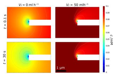
Fig. 11 Typical simulated concentration profiles showing the cross-section of the electrode for (left) region A,  $V_f = 0$  ml h<sup>-1</sup>, and (right) region B,  $V_f = 50$  ml h<sup>-1</sup>, at t = 0.1 (top) and 30 s (bottom). The white bar in the centre of each image shows the membrane with the FcMeOH depletion originating from the right-hand side of the nanoband. Flow is again from bottom to top in the right-hand images.
