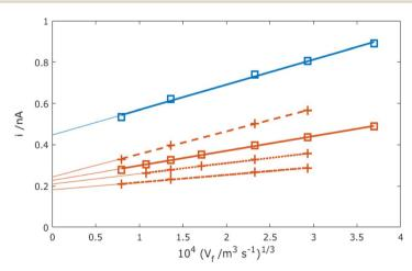
Fig. 12 Simulated currents at a single nanoband against  $V_{\rm f}^{1/3}$  over the linear region with linear regression lines and extrapolated to zero flow. Simulations are for  $D=1.43\times 10^{-9}$  m<sup>2</sup> s<sup>-1</sup> (blue) and  $D=0.7\times 10^{-9}$  m<sup>2</sup> s<sup>-1</sup> (red) at  $x_{\rm E}=50$  nm (solid line, squares), and  $x_{\rm E}=10$  (dot-dash line), 25 (dotted line) and 100 nm (dashed line) for  $D=0.7\times 10^{-9}$  m<sup>2</sup> s<sup>-1</sup>.
