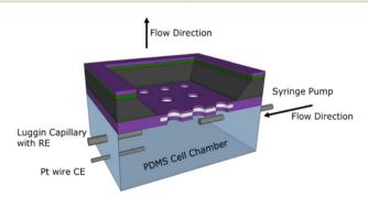
Fig. 4 The flow test-cell configuration, showing the electrodes and syringe pump connection, flow directions and MNE device orientation. Note that the MNE array has the back-side orientation uppermost. Also shown are the electrode (grey) and membrane insulator (purple) layers.
