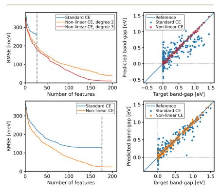
Fig. 5 Left: fitting errors for standard (blue) and nonlinear CE models (orange and red) based on a pool of 27 clusters (top) and 176 clusters (bottom). Right: predicted *versus* target bandgaps for the standard CE with 27 clusters and the nonlinear CE of degree 3 models with 150 features (top), and standard CE and nonlinear CE models with 150 clusters/features (bottom).
