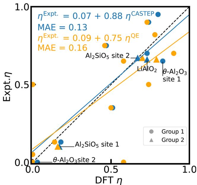
Fig. 2 Reference scale for  $^{27}\text{Al}$   $\eta$ . The  $^{27}\text{Al}$   $\eta$  values for 15 Al-containing compounds are simulated with PBE, fixed cell geometries, default PP, and unit cells using CASTEP (blue) and Quantum ESPRESSO (orange). The experimental values from literature can be found in ESI Table S3. †  $\kappa\text{-Al}_2\text{O}_3$  and  $\text{AlVO}_4$  are omitted (see text). The dashed diagonal line indicates the limit of ideal correlation.
