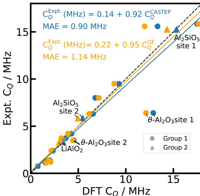
Fig. 1 Reference scale for  $^{27}\text{Al } C_Q$ . The  $^{27}\text{Al } C_Q$  values for 15 Al-containing compounds are simulated with PBE, fixed cell geometries, default PP, and unit cells using CASTEP (blue) and Quantum ESPRESSO (orange). The experimental values from literature can be found in ESI Table S3.†  $\kappa\text{-Al}_2\text{O}_3$  and  $\text{AlVO}_4$  are omitted (see text). The dashed diagonal line indicates the limit of ideal correlation.
