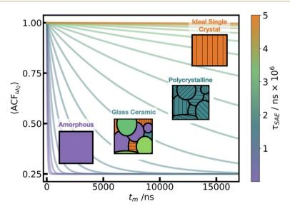
Fig. 7 Schematic of range of crystalline to amorphous  $\tau_{SAE}$ . The plot shows a range of decay functions, eqn (5), with  $\tau_{SAE}$  from 50 ns to 5 million ns. The inset figures show schematics of the expected microscale structure at each of these varying decay rates, with black lines in the glass ceramic and polycrystalline denoting different grains.
