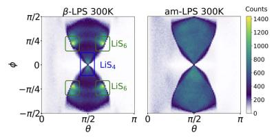
Fig. 6 Heatmap  $\theta$  and  $\phi$  distributions in β- and am-LPS. The heatmaps show the concentration of the angles  $\theta$  and  $\phi$  across the full 1  $\mu$ s UFP-MD trajectory. The distributions are colored by the total number of sites with that combination of angles ( $\theta$ ,  $\phi$ ), and in β-LPS the angle pairs which arise from LiS<sub>4</sub> and LiS<sub>6</sub> sites are indicated.
