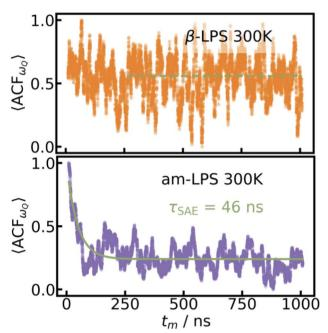
Fig. 3  $\langle ACF_{\omega_0} \rangle$  for  $\beta$ -LPS and am-LPS. The  $\langle ACF_{\omega_0} \rangle$  given by eqn (4) calculated over a 1  $\mu$ s UFP-MD simulation at 300 K for 144 Li atoms in single-crystalline  $\beta$ -LPS (top, orange) and 216 Li atoms in am-LPS (bottom, purple). A decay time,  $\tau_{SAE} = 46$  ns, can be extracted from the am-LPS  $\langle ACF_{\omega_{\alpha}} \rangle$ .
