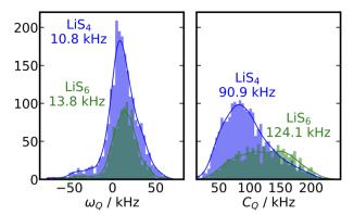
Fig. 4 Distributions of  $ω_Q$  and  $C_Q$  in β-LPS. The left panel shows the distribution of tetrahedral LiS<sub>4</sub> sites (blue) to octahedral LiS<sub>6</sub> sites (green), calculated using DFT, for the crystalline β-LPS structure. The right panel uses the same color scheme to show the distributions of  $C_Q$  sites for β-LPS.  $C_Q$  and  $ω_Q$  are calculated for all 33 β-LPS structures in the ML-EFG model.
