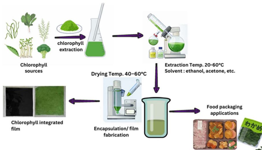
Fig. 2 Schematic of chlorophyll-based active film synthesis. 46,47
