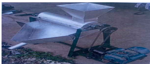
Fig. 2 Assembled motorized cashew apple juice extraction machine.
