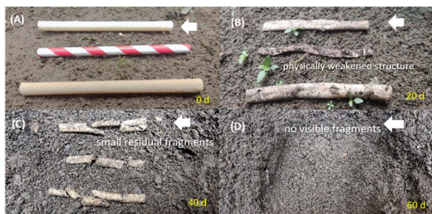
Fig. 10 Degradability testing of selected low-speed S-B9 straws, commercial plastic-coated paper straw, and high-speed S-B9 straws (from bottom to top): (A) 0 days after burial in soil; (B) 20 days after burial; (C) 40 days after burial; (D) 60 days after burial.
