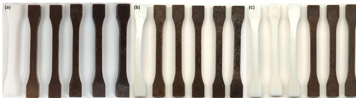
**Fig. 1** Injection-molded dog bone specimens of (a) PBS and its composites containing 30, 40, 50, 60, and 70 wt% potato peels (PP); (b) PBAT and its composites with 30, 40, 50, 60, and 70 wt% PP; and (c) PBS/PBAT blends with mass ratios of 70/30, 50/50, and 30/70, each containing 30 wt% PP.
