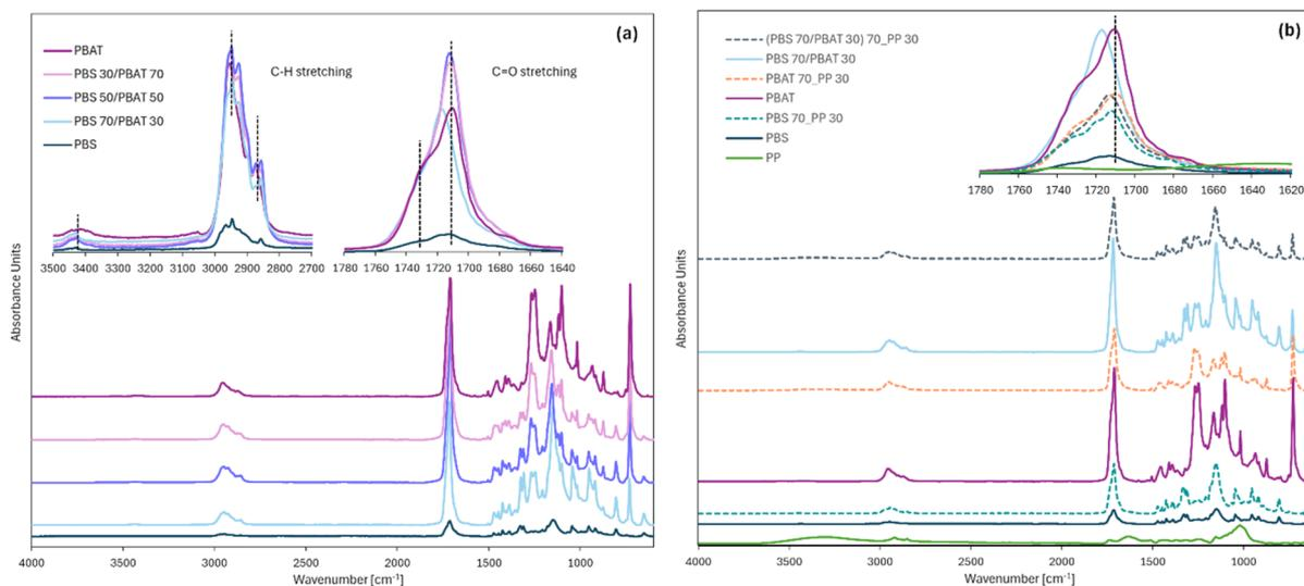
**Fig. 2** FTIR absorption spectra of (a) neat PBS, PBAT and their blends, and (b) potato peels (PP) and its composites with PBS, PBAT and the blend PBS 70/PBAT 30 at 30 wt% PP content, measured in the range of  $600\text{--}4000\text{ cm}^{-1}$ .
