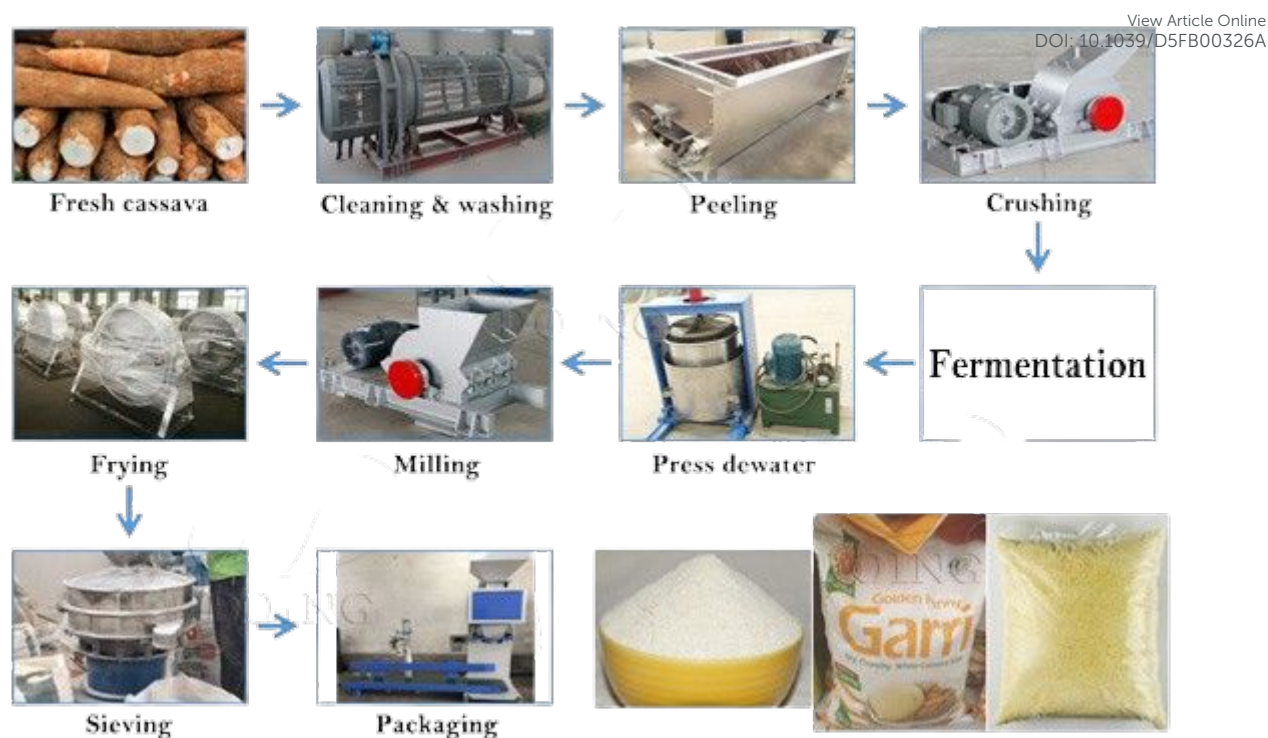
Figure 4. Mechanised gari production process diagram. 126
