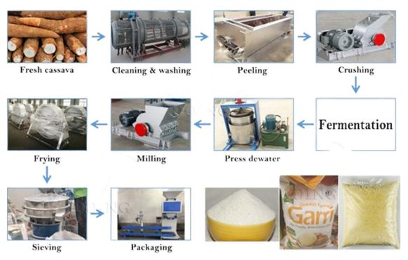
Fig. 4 Mechanised gari production process diagram. 125
