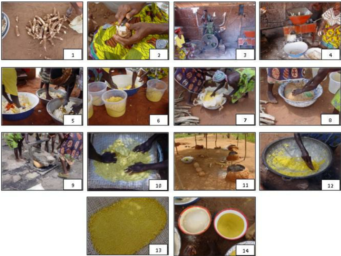
Fig. 3 The artisanal gari production process. 122 (1) Cassava tubers after harvesting, (2) tubers are peeled and washed, (3) mechanical grinding of the tubers, (4) collection of the ground tubers, (5) palm oil and soy bean added, (6) placed in buckets, sealed with lids, and left to ferment for 48 h, (7) and (8) mixture is placed in a large bag, (9) the dewatering process, (10) sieving to remove large particles, (11) area where mixture is fried/garified, (12) frying/garification, (13) fine sieving, and (14) comparison between traditional gari (left) and gari fortified with soybean and palm oil.
