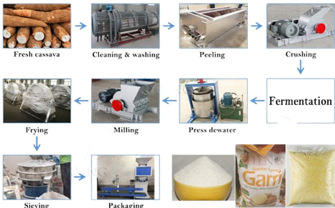
Fig. 4 Mechanised gari production process diagram. 125
