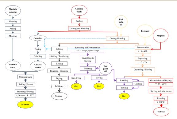
Fig. 2 Schematic diagram of the production process of some types of semolina made from the roots (cassaya) and plantain.
