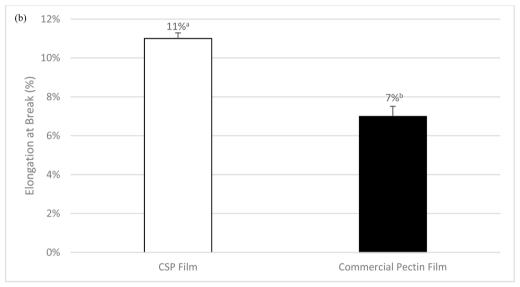
Fig. 4 Comparison of the preliminary mechanical properties of CSP film and commercial pectin film. (a) Tensile strength, (b) elongation at break. Different superscript letters indicate a significant difference (p < 0.05).
