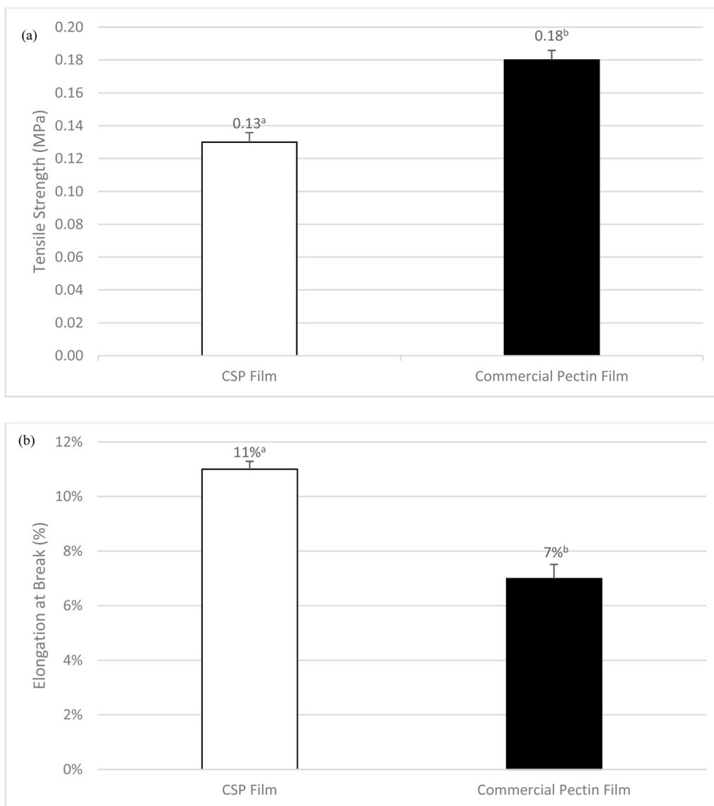
Fig. 4 Comparison of the preliminary mechanical properties of CSP film and commercial pectin film. (a) Tensile strength, (b) elongation at break. Different superscript letters indicate a significant difference ( $p < 0.05$ ).
