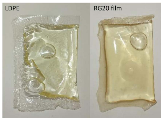
Fig. 3 Photographs of soybean oil packaged in the RG20 film and LDPE pouches.
