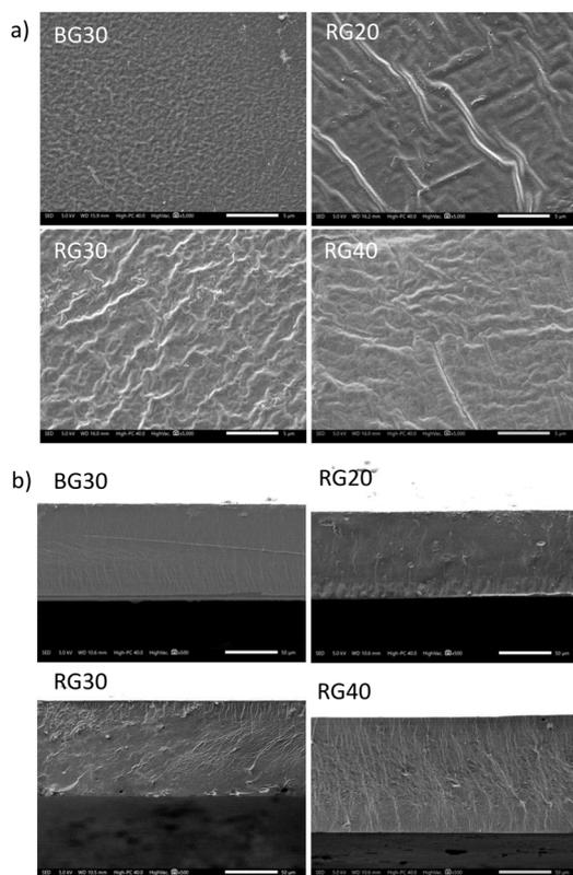
Fig. 2 SEM micrographs of the surface (a) and cross-section (b) of edible films with different glycerol concentrations.
