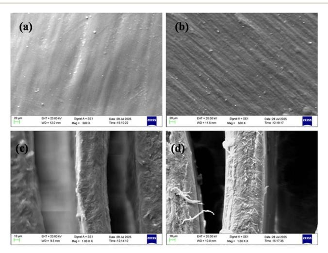
Fig. 2 SEM images of (a) PLA/PBAT blend control film and (b) PLA/PBAT blend + 4 wt% ε-PL film. (c) Cross-sectional image of the PLA/PBAT blend control film. (d) Cross-sectional image of the PLA/PBAT blend + 4 wt% ε-PL film.
