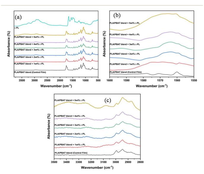
Fig. 1 (a) FTIR spectra of ε-PL, PLA/PBAT blend control film and PLA/PBAT blend films loaded with different weight percentages of ε-PL (1–5 wt%). (b) Enlarged view of the FTIR spectra in the 1550-1600 cm<sup>-1</sup> regions. (c) Enlarged view of the FTIR spectra in the 2800-3500 cm<sup>-1</sup> regions.
