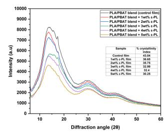
Fig. 5 XRD graph of the PLA/PBAT blend control film and PLA/PBAT blend loaded films with different weight percentages of  $\varepsilon$ -PL (1–5 wt%).
