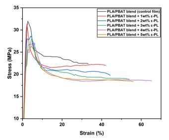
Fig. 6 Stress-strain curve of the PLA/PBAT blend control film and PLA/PBAT blend films loaded with different weight percentages of  $\varepsilon$ -PL (1-5 wt%)
