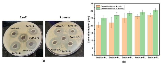
Fig. 7 (a) Antimicrobial activity of PLA/PBAT blend films loaded with different weight percentages of ε-PL (1–5 wt%) using film extract (200 μL) evaluated by the well diffusion assay and incubated at 37 °C for 24 h. (b) Zone of inhibition bar graph of PLA/PBAT with  $\varepsilon$ -PL (1–5 wt%) film extract against E. coli and S. aureus.
