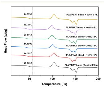
Fig. 4 DSC thermogram of the PLA/PBAT blend control film and PLA/PBAT blend films loaded with different weight percentages of ε-PL (1-5 wt%).
