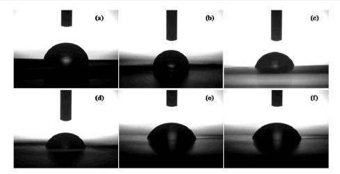
Fig. 3 Image of droplets formed on the surface of (a) PLA/PBAT blend control film, (b) PLA/PBAT blend + 1 wt%  $\epsilon$ -PL film, (c) PLA/PBAT blend + 2 wt%  $\epsilon$ -PL film, (d) PLA/PBAT blend + 3 wt%  $\epsilon$ -PL film, (e) PLA/PBAT blend + 4 wt%  $\epsilon$ -PL film, and (f) PLA/PBAT blend + 5 wt%  $\epsilon$ -PL film.
