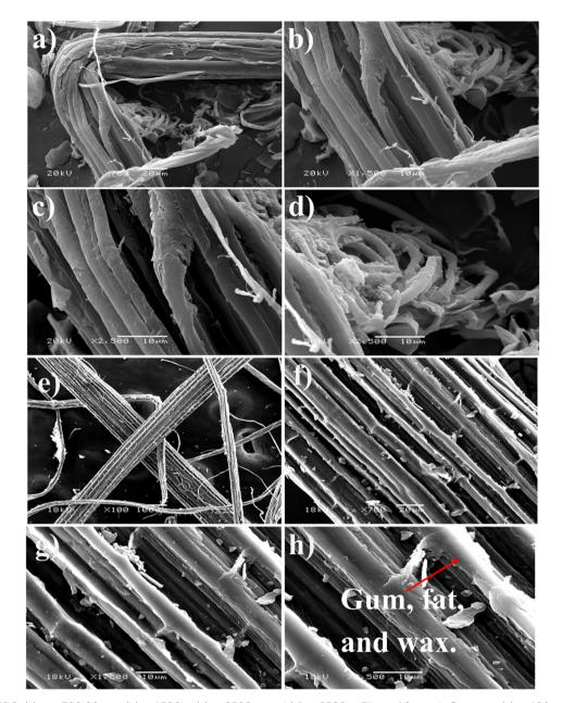
Fig. 3 Fiber of MD2: (a) at  $\times$ 700 20  $\mu$ m, (b) at 1500 $\times$ , (c) at 2500 $\times$ , and (d) at 2500 $\times$ . Fiber of Smooth Cayenne: (e) at 100 $\times$ , (f) at 700 $\times$ , (g) at 1500 $\times$ , and (h) at 2500 $\times$ .
