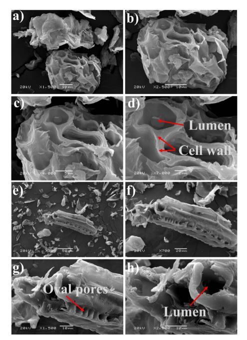
Fig. 2 Powder of MD2: (a) at  $1500 \times$ , (b) at  $2500 \times$ , (c) at  $4000 \times$ , and (d) at  $7000 \times$ . Powder of Smooth Cayenne: (e) at  $350 \times$ , (f) at  $700 \times$ , (g) at  $1500 \times$ , and (h) at  $2500 \times$ .
