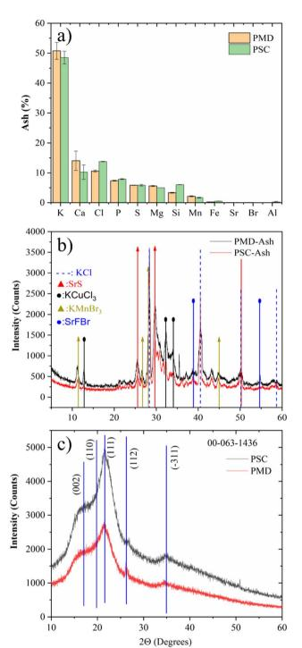
Fig. 4 (a) Concentration of minerals in ash powder of MD2 (PMD) and Smooth Cayenne (PSC). (b) X-ray diffraction patterns of the PMD-Ash (MD2 - ash powder) and PSC-Ash samples: (Cayena Lisa - ash powder). (c) X-ray diffraction patterns of PMD (MD2 powder) and PSC (Smooth Cayenne powder) samples
