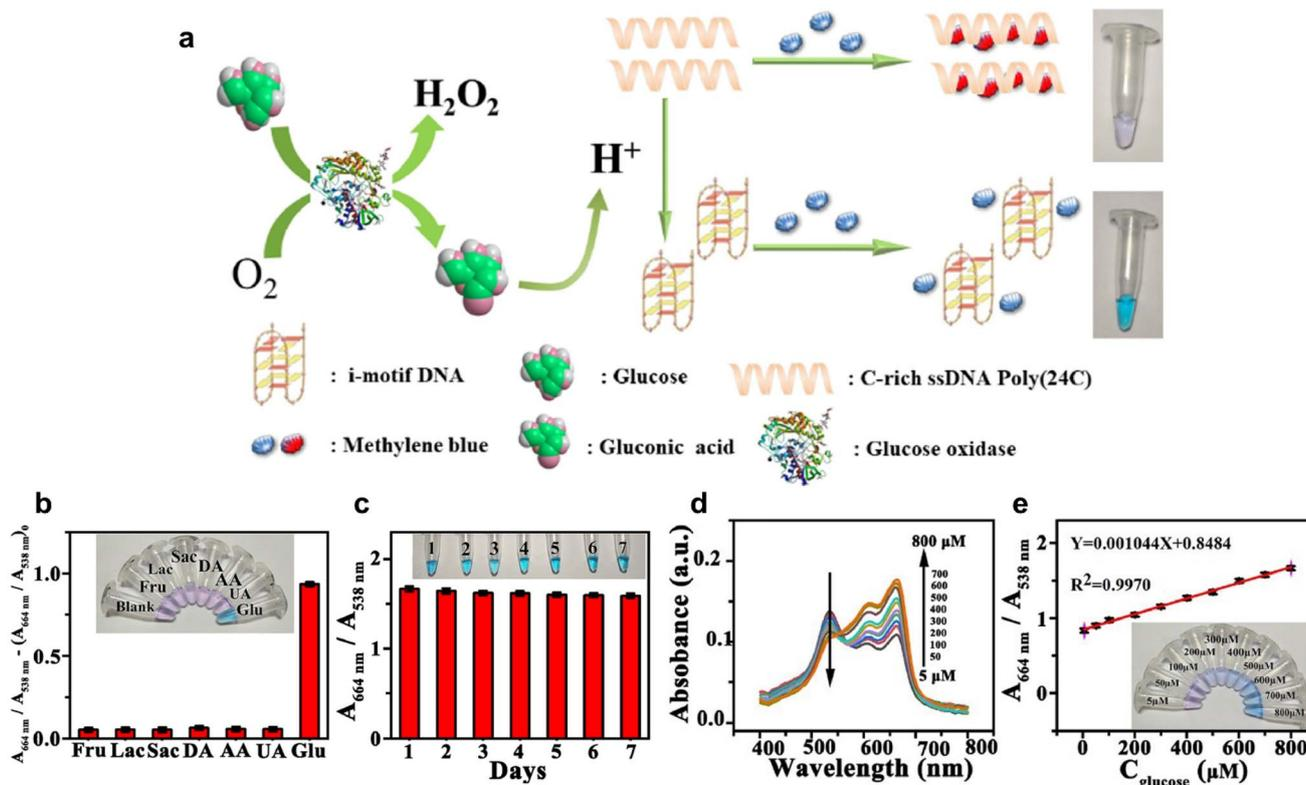
Fig. 9 Colorimetric and ratiometric glucose detection based on pH-sensitive i-motif DNA. (a) Schematic of glucose detection mechanism using  $GO_x$  and i-motif DNA (Poly(24C)). (b) Selectivity test for glucose against interferents. (c) Sensor stability over seven days. (d) and (e) UV-vis spectra and calibration curve demonstrating linear response to glucose concentrations ( $R^2 = 0.997$ ). Reproduced with permission from ref. 24 Copyright 2020, Elsevier.
