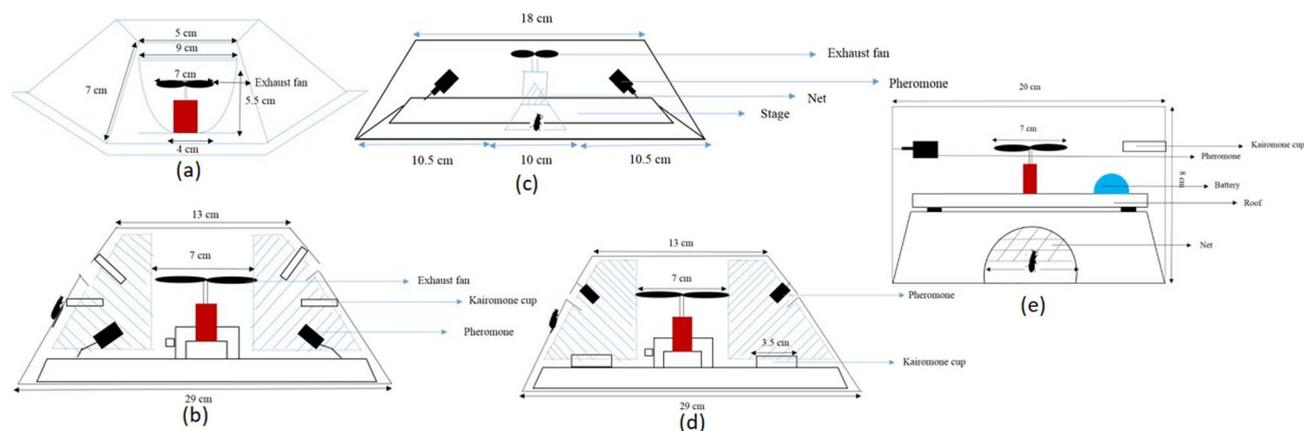
Fig. 2 Pitfall style dome traps which have a hexagonal shape (a), triangular shape (b–d) and square shape (e).<sup>39</sup>
