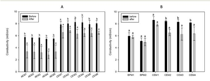
Fig. 6 Membrane conductivity before and after (A) ED and (B) EDBM. Different letters indicate significant differences between the means (Tukey, p < 0.05).
