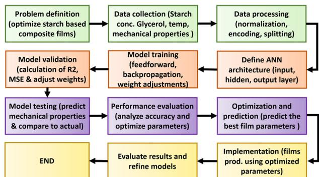
Fig. 4 Flow chart for artificial neural networks.
