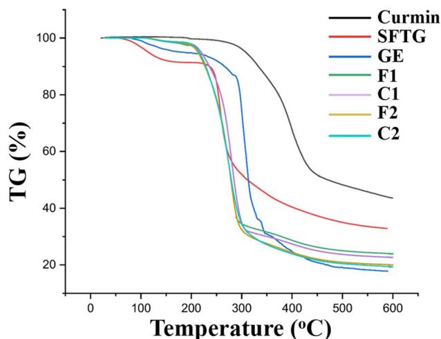
Fig. 9 Thermogravimetric analysis (TGA) of pure curmin, SFTG, GE, and several film formulations (F1, F2, C1, and C2).<sup>91</sup> Adapted from open access under the Creative Commons BY license. Copyright 2022 MDPI.
