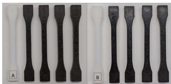
Fig. 5 Injection-moulded dog-bone specimens made of neat PBS (A) or PBAT (B) and their respective composites containing 30, 40, 50 and 60 wt% milled spent coffee grounds (SCG_m).
