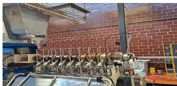
Fig. 1 Twin-screw extruder.
