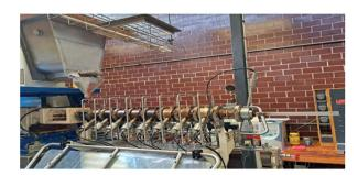
Fig. 1 Twin-screw extruder.
