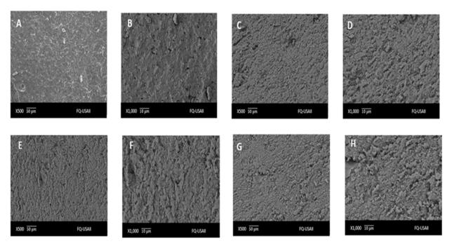
Fig. 6 Images of the extruded analogues: (A and B) SPI + AO; (C and D) SPI + AO + 2% by weight of pectin; (E and F) SPI + AO + 4% by weight of pectin; (G and H) SPI + AO + 6% by weight of pectin.
