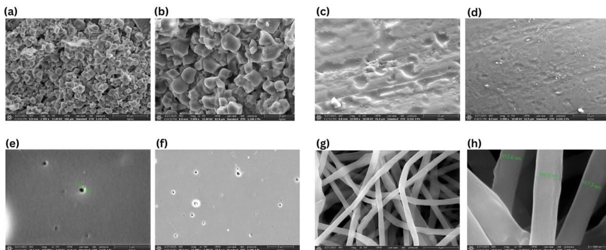
Fig. 3 SEM micrographs of 3D-printed edible cups: an (a and b) uncoated porous matrix (ragi/sago base), (c and d) zein spray-coated edible cup surface (smoother morphology), (e and f) high-res zein film nanostructure showing a dense network, and (g and h) zein nanofiber network (scale bars: a and b: 40–20  $\mu$ m, c and d: 10–20  $\mu$ m, e and f: 1–5  $\mu$ m, and g and h: 4  $\mu$ m–500 nm).
