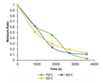
Fig. 2 Drying kinetics of convective-dried foam-mat chokeberry pulp at various temperatures (50, 60, and 70 °C).
