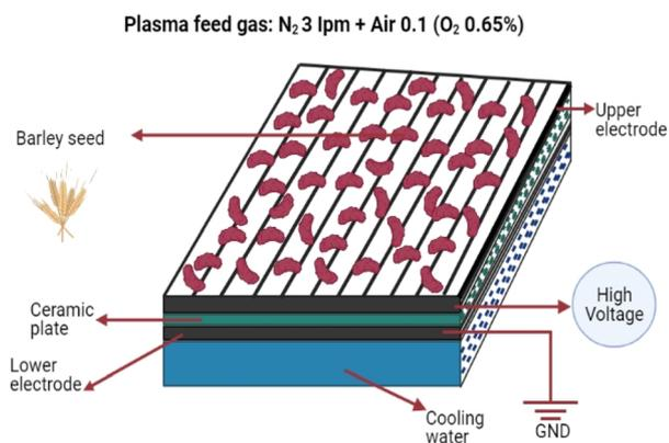
Fig. 4 Surface dielectric barrier discharge plasma treatment.<sup>199</sup>
