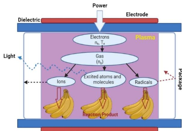
Fig. 1 In-package cold plasma treatment.<sup>40</sup>
