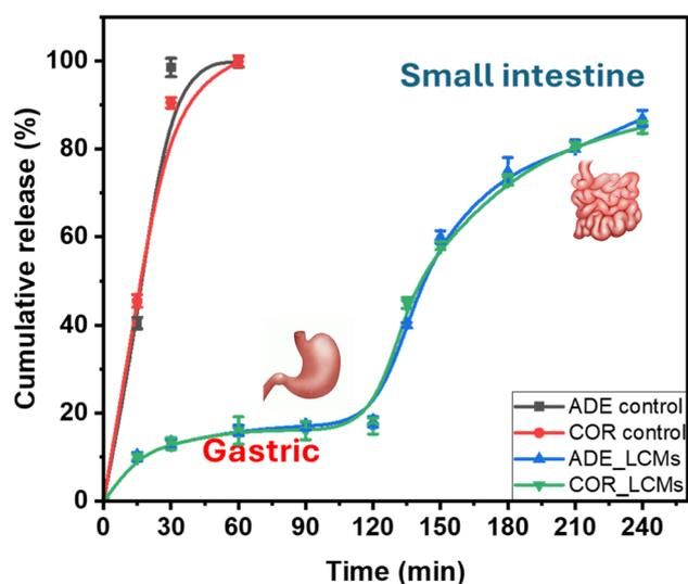
Fig. 5 Cumulative release curves of ADE and COR from extract and LCMs during *in vitro* gastrointestinal digestion simulated at 37 °C (where squares and circles represent the release of ADE and COR from the extract (control), and triangles represent the release from LCMs).
