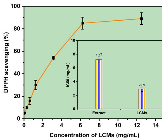
Fig. 4 DPPH free radical scavenging activity of the LCMs system at various concentrations, along with the IC<sub>50</sub> values of the LCMs system compared to the extract.
