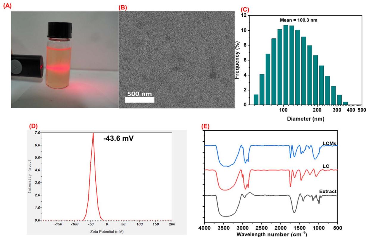
Fig. 2 Characteristics of the LCMs, (A): Photograph of the LCMs sample demonstrating the Tyndall effect (diluted with water at a 1 : 10 ratio), (B): morphology of LCMs particles observed using Transmission Electron Microscopy (TEM), (C): particle size distribution by DLS, (D): zeta potential, (E): FTIR spectra of the individual components and the LCMs system.
