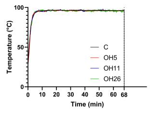
Fig. 2 Thermal profile of wort boiling under different heating conditions: conventional (C) boiling represented in black, ohmic heating (OH) boiling at 4-5 V cm<sup>-1</sup> (OH5) represented in red. OH boiling at 8-11 V cm $^{-1}$  (OH11) represented in blue, and OH boiling at 22–26 V cm $^{-1}$ (OH26) represented in red.
