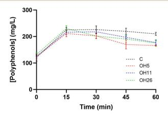
Fig. 5 Evolution of polyphenol concentration (mg L<sup>-1</sup>) in wort samples monitored at 15-minute intervals, over a 60-minute boiling period. Boils were performed through conventional (C) heating, in black, and ohmic heating (OH) methods using different electric field intensities:  $4-5 \text{ V cm}^{-1}$  (OH5) in red,  $8-11 \text{ V cm}^{-1}$  (OH11) in blue, and 22-26 V cm $^{-1}$  (OH26) in green. Points represent mean values  $\pm$ standard deviation (n = 3), presented in Table S3.
